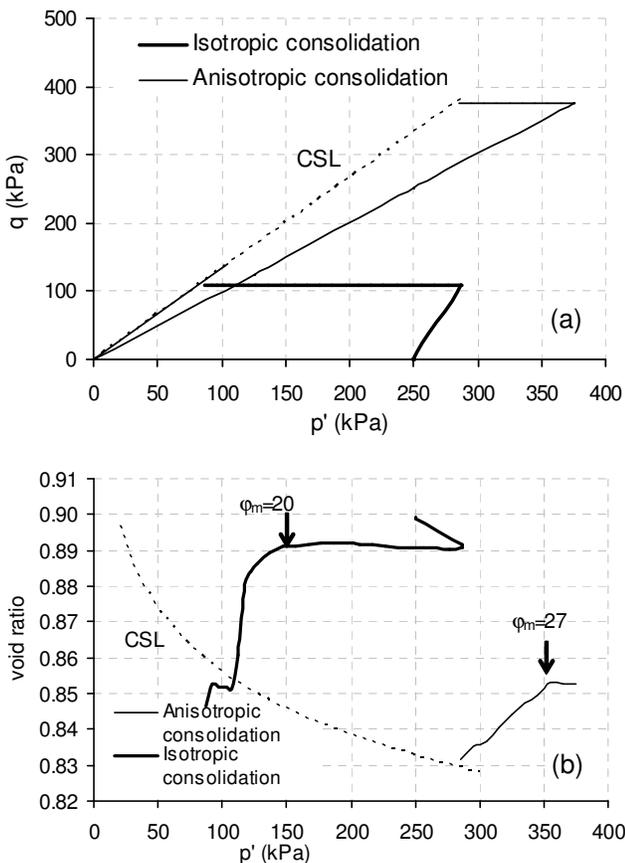
Figure 7. Effect of anisotropic consolidation: (a) stress path (b) variation of void ratio with mean normal stress.
