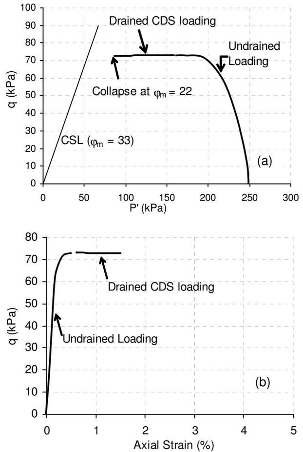
Figure 4. Behavior of saturated sand in CDS loading: (a) Stress path (b) Deviatoric stress v.s. axial strain.
