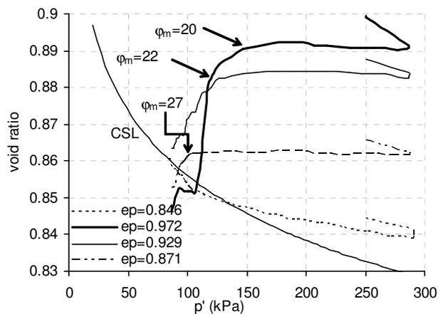
Figure 5. Effect of void ratio on the potential for volume contraction in CDS loading.
