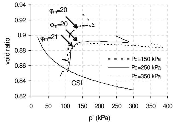
Figure 6. Effect of confining pressure on sand behavior in the CDS loading.
