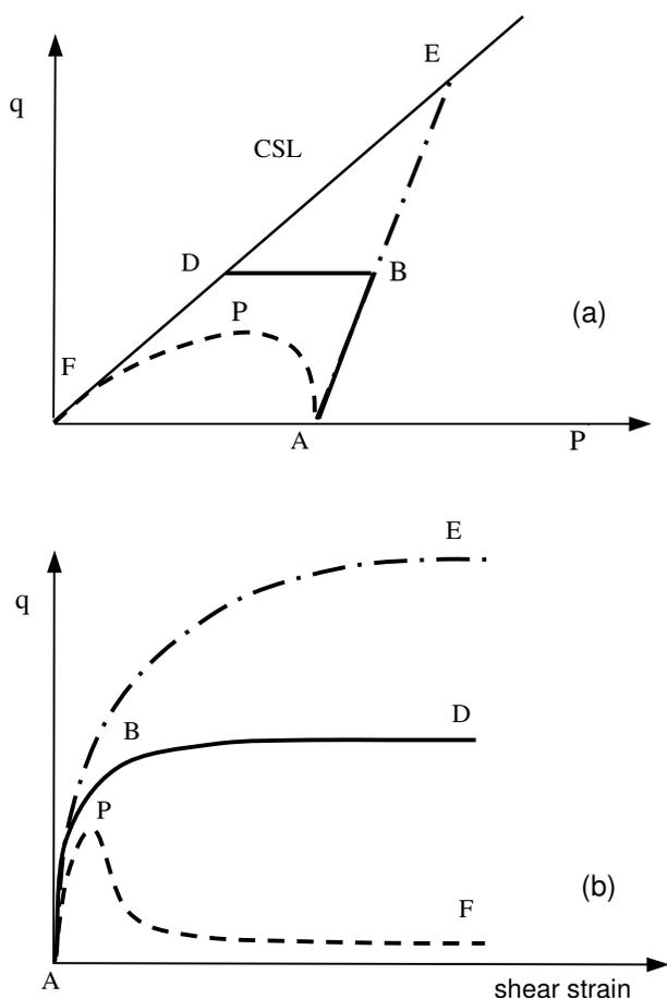
Figure 1. Typical results of tests on very loose sand
