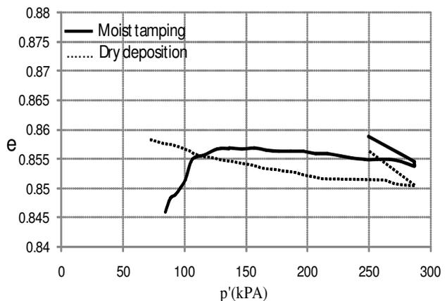
Figure 8. Behavior of moist tamped and dry deposited sand subjected to CDS loading
