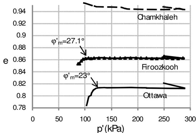
Figure 9. Behavior of three different sands with the same relative density, subjected to the same CDS stress path
