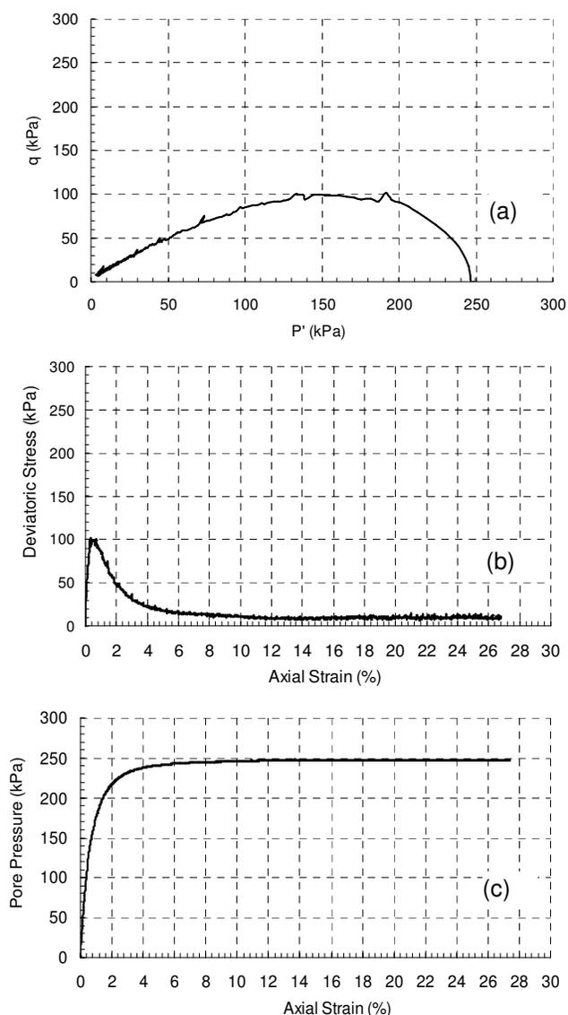
Figure 2. Results of undrained test on very loose Firoozkooh sand (a) stress path (b) stress-strain relationships (c) pore pressures generated
