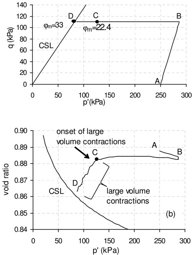
Figure 3. Typical behavior of dry sand in CDS loading: (a) stress path; (b) changes in void ratio
