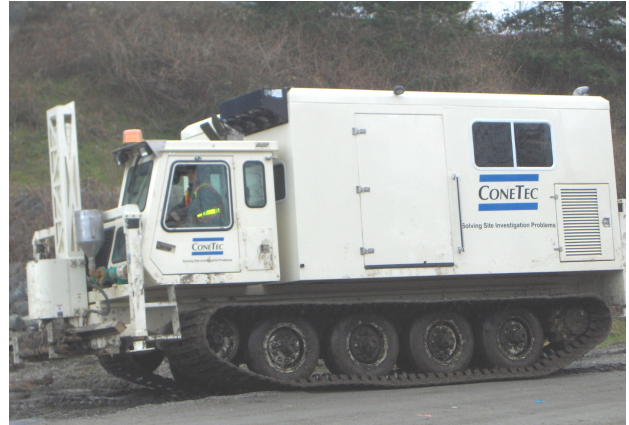
Figure 2. Typical ConeTec Track Mounted Rig Used at Fort McMurray Sites.
