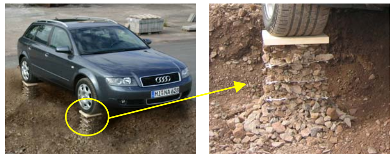
Figure 3. Lateral restraint of aggregate using high modulus laid and welded geogrids
