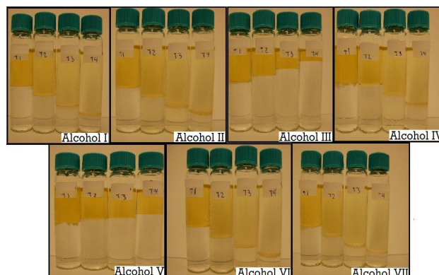
Figure 8. Initial mixtures for tie lines construction for alcohols types
