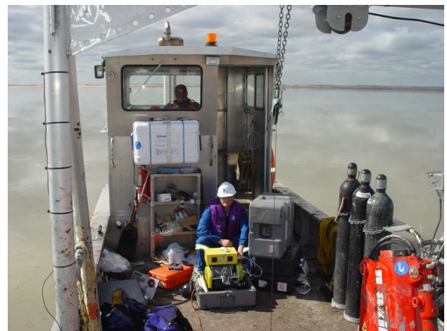
Photo 1. Geophysical logging setup on barge at tailings pond facility.
