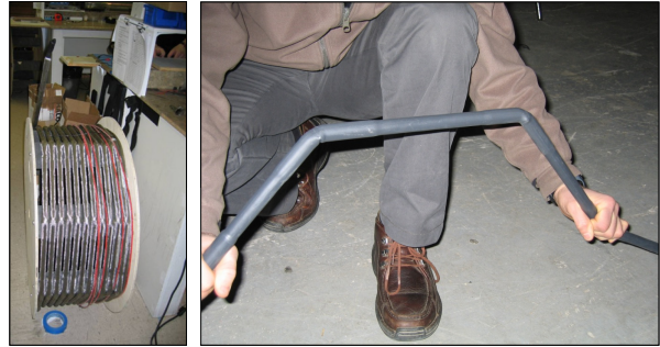
Figure 4. Left: SAA on reel. Right: SAA rigid segments connected by joints that resist twist. Segments hold MEMS accelerometers, microprocessors, and electronics.
