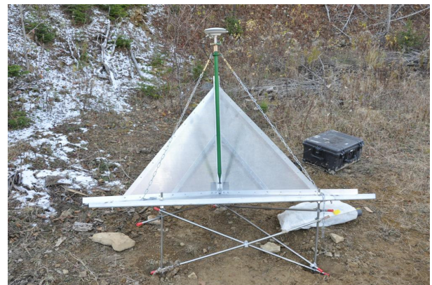
Figure 4. Photo of a corner reflector (CR1) installed at the Gascons site. A D-GPS antenna is temporarily
