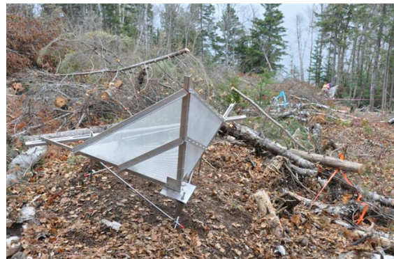
Figure 9. Photo of corner reflector CR5 located on the north side of fissure No.G.
