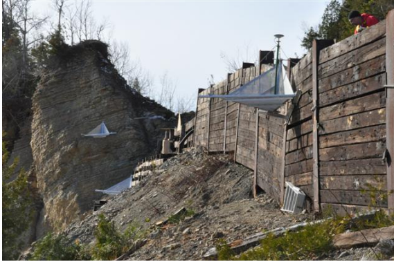
Figure 11. Photo illustrating corner reflector CR7 (foreground) with a D-GPS unit mounted on it. Corner reflector CR8 installed on the retaining wall (left-hand side of the photo) and CR3 anchored on a southeast face of the Petit-massif (background).
