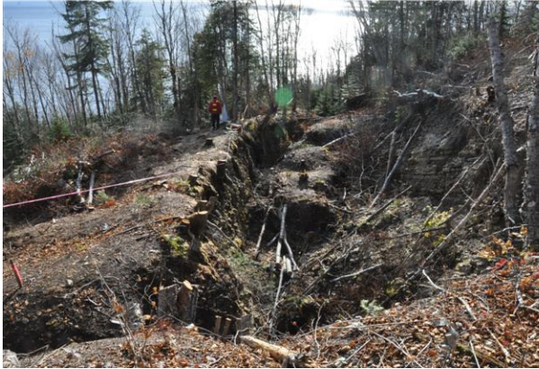
Figure 3. Photo illustrating a large open fissure in the forested sector (Sector II in Figure 2) above the railway corridor.
