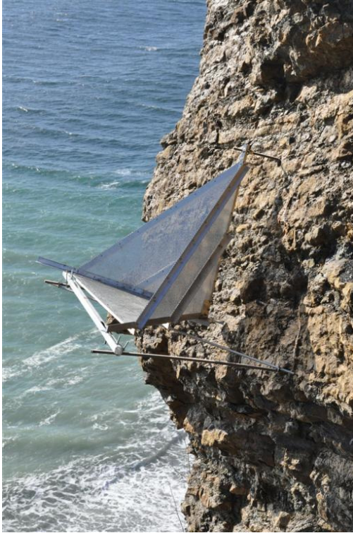
Figure 7. Corner reflector CR3 anchored on a southeast facing rock face of the Petit-massif at the Gascons site.
