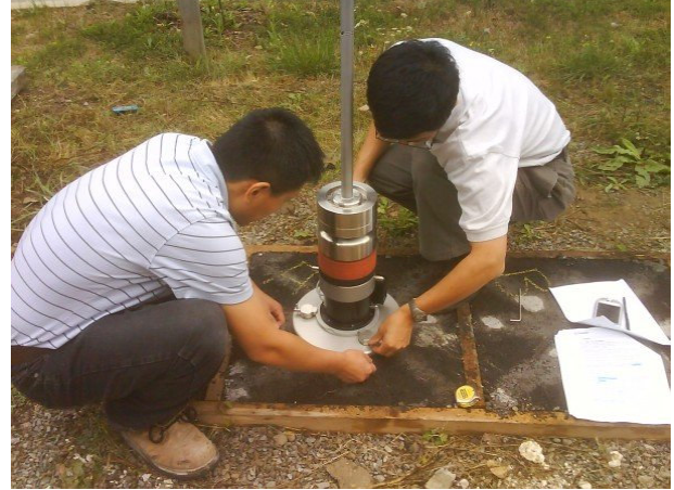
Figure 4. Site layout showing base and LWD test set up.
