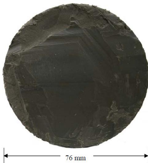
Figure 4. Photograph of a typical core sample extruded from Denison core barrel.
