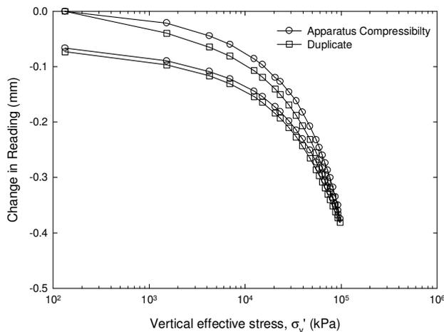
Figure 6. Compressibility of oedometer apparatus.
