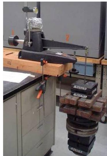
Figure 5. Photograph of oedometer apparatus.
