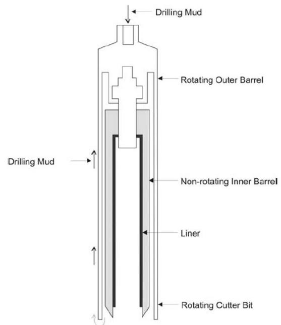
Figure 2. Schematic of Denison core barrel (modified from Terzaghi et al., 1996).
