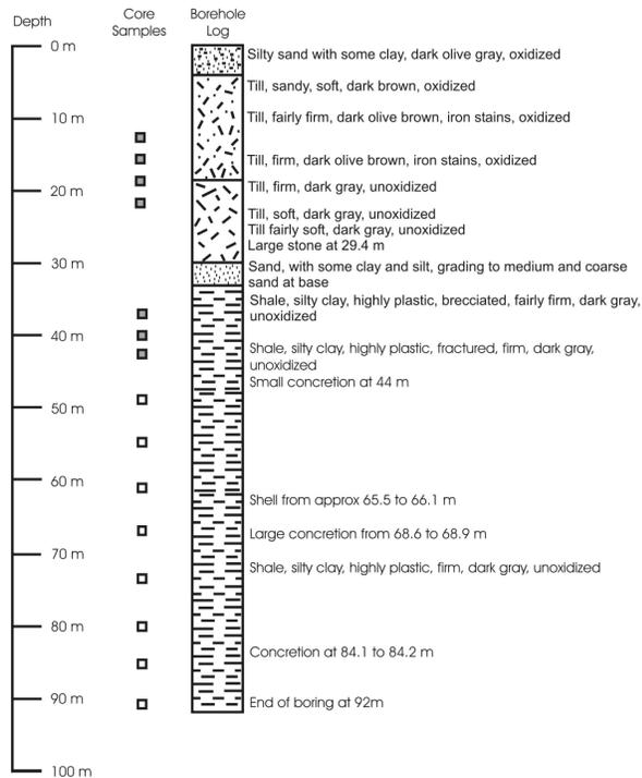
Figure 3. Stratigraphic log and collected core samples. Shaded squares are Shelby tubes, open squares are Denison core barrels.
