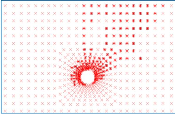
Figure 7. Failure mechanism of surrounding soil with  $\alpha=15^\circ$
