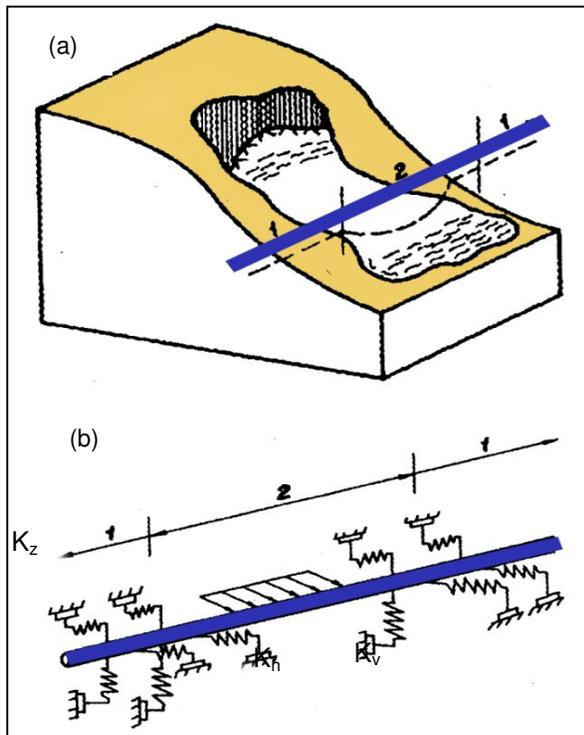
Figure 1. (a) Pipeline displacement due to PGD, (b) Winkler type spring soil-pipe model (Winkler, 1867)
