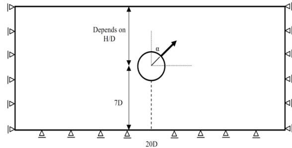
Figure 2. Schematic of a buried pipe
