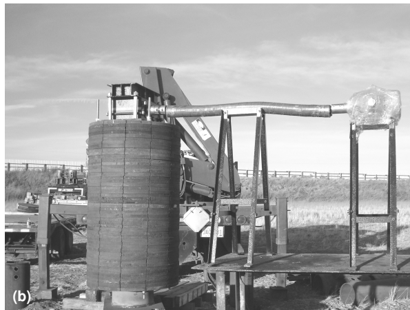
Figure 4. Dynamic testing; (a) horizontal vibration; (b) vertical vibration
