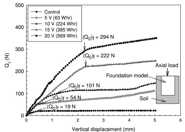
Figure 7. Axial load capacity,  $Q_c$ , vs. vertical displacement of the foundation model – test series 2 ( $\beta = 1$ )
