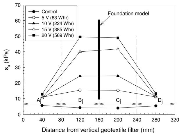
Figure 11. Undrained shear strength,  $s_u$ , across the cell - test series 2 ( $\beta = 1$ )
