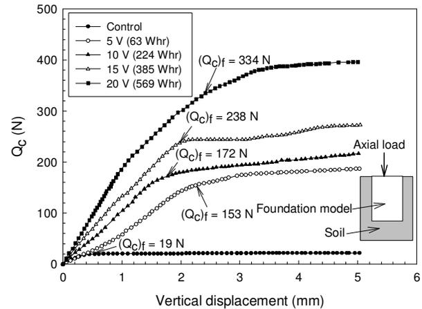
Figure 6. Axial load capacity,  $Q_c$ , vs. vertical displacement of the foundation model – test series 1 ( $\beta = 0.5$ )
