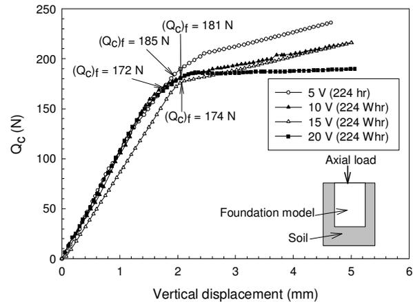
Figure 9. Axial load capacity,  $Q_c$ , vs. vertical displacement of the foundation model – test series 3
