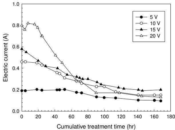
Figure 3. Electric current vs. cumulative treatment time – test series 1 ( $\beta = 0.5$ )
