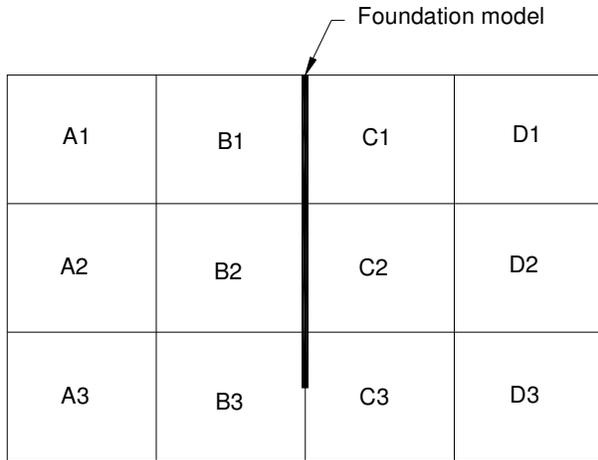
Figure 2. Locations of water content and undrained shear strength,  $s_u$ , measurements after the triaxial loading
