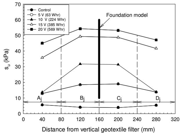
Figure 10. Undrained shear strength,  $s_u$ , across the cell - test series 1 ( $\beta = 0.5$ )
