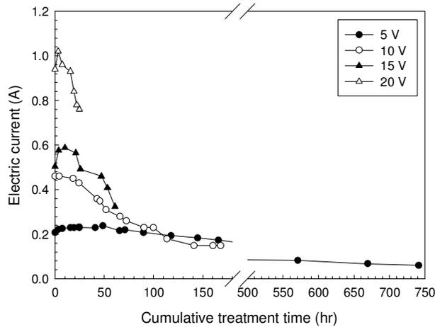
Figure 5. Electric current vs. cumulative treatment time – test series 3 ( $\beta = 0.5$ )
