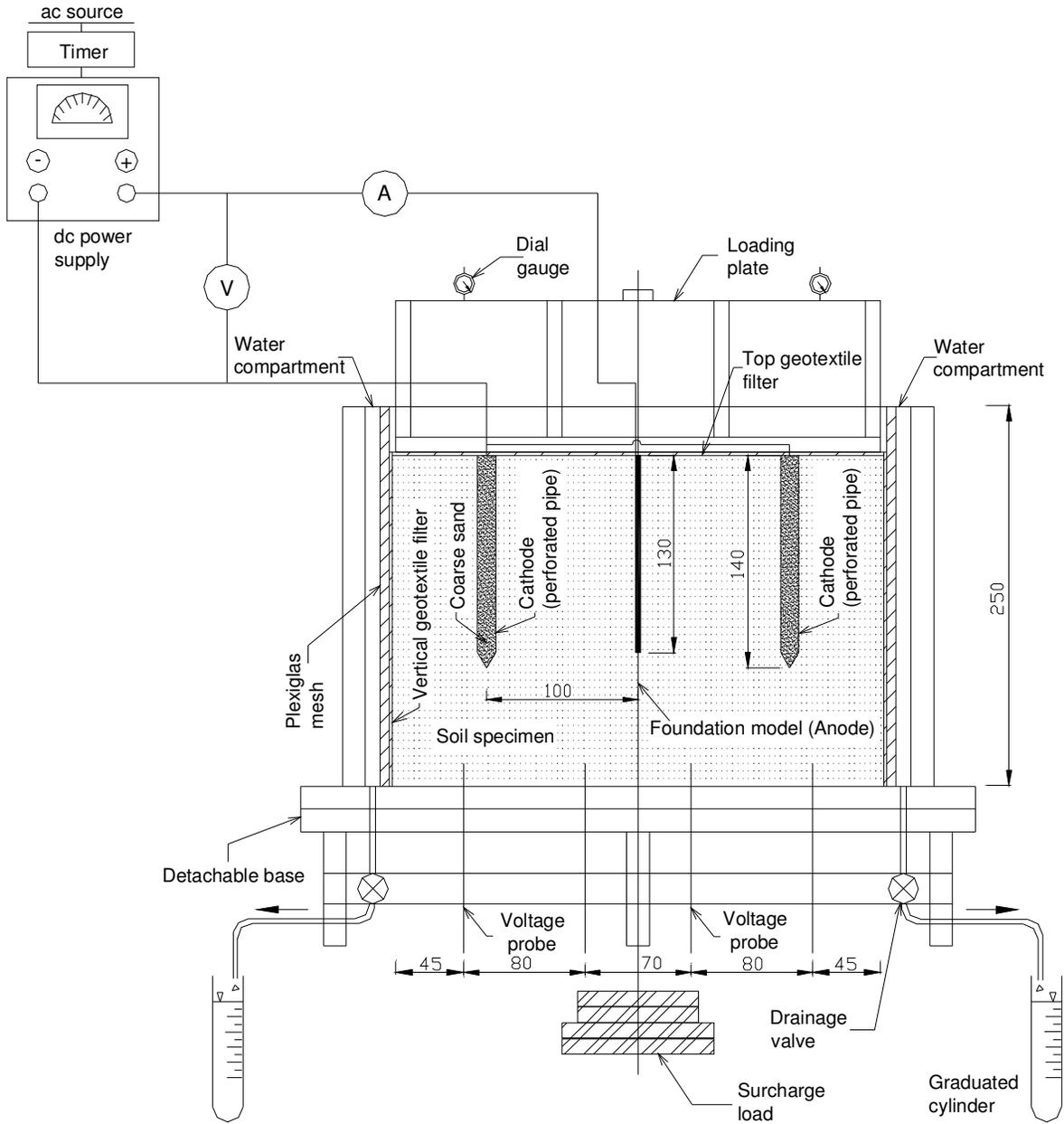
Figure 1. Elevation view of electrokinetic treatment cell
