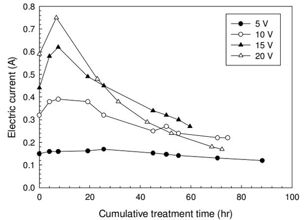
Figure 4. Electric current vs. cumulative treatment time – test series 2 ( $\beta = 1$ )
