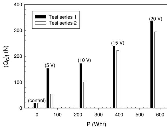
Figure 8. Axial load capacity at failure,  $(Q_c)_f$ , vs. energy consumption, P for test series 1 and test series 2
