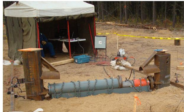
Figure 3. Typical lateral load test setup
