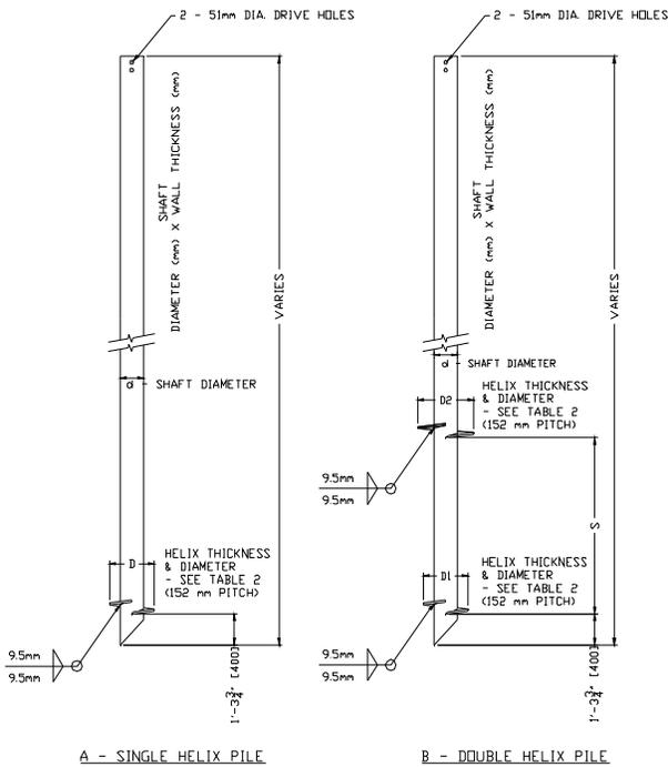
Figure 1. Typical helical pile configuration
