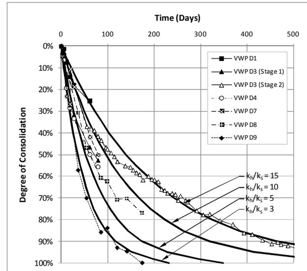
Figure 3. Results of Back Analysis for Six VWPs in Swamp 'D'
