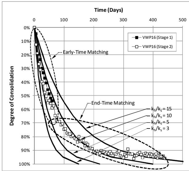
Figure 5. Comparison of early-time and end-time Matching for VWP16 in Swamp '605'
