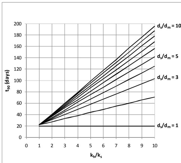
Figure 2. Effect of Smear Ratio ( $k_h/k_s$ ) on Time for 90% Horizontal Consolidation
