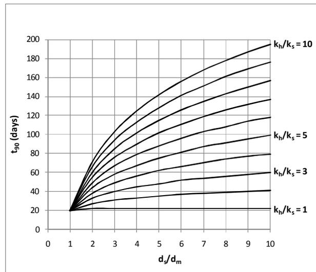
Figure 1. Effect of Diameter of Smear Zone ( $d_s$ ) on Time for 90% Horizontal Consolidation
