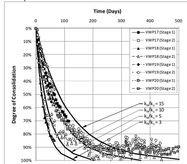
Figure 4. Results of Back Analysis for Four VWPs in Swamp '605'
