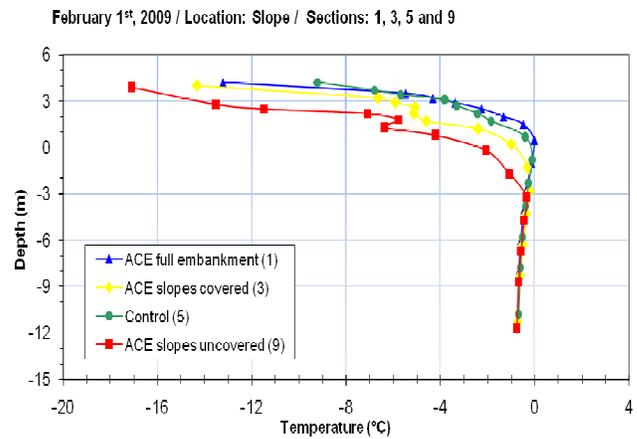
Figure 5: Thermal regimes in air convection embankment sections compared with the control section (February 1<sup>st</sup>, 2009)
