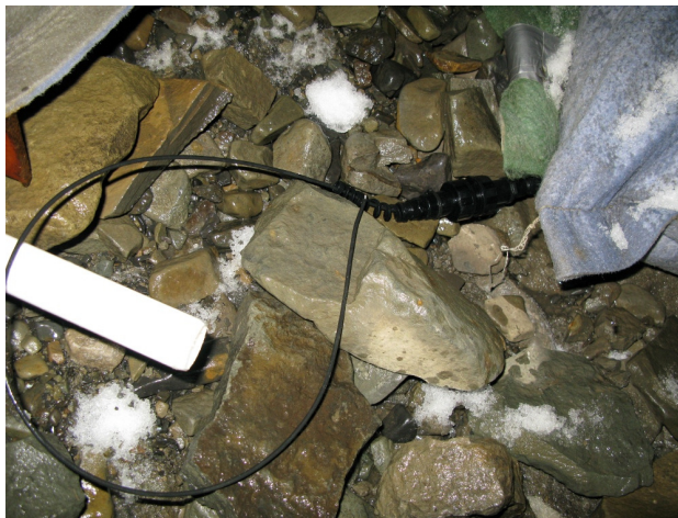
Figure 13. The connection cable from the textile fiber optic sensing strip below the geobags.
