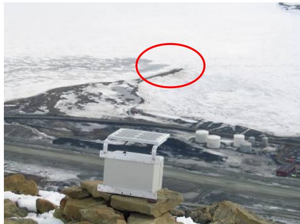
Figure 9. Time lapse camera on Liljevalchjellet above Svea taking pictures of the sea ice in Sveasundet, May 22nd 2007. The experimental breakwater in the red circle (Caline, 2010)
