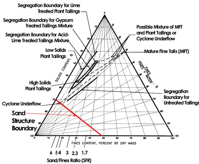
Figure 6. Segregation boundary diagram.
