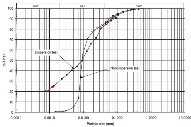
Figure 5. Dispersed and nondispersed PSD.
