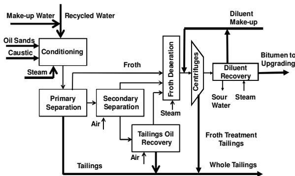
Figure 1. CHWE process schematics.
