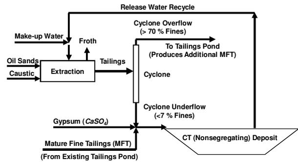
Figure 2. Production of Composite Tailings (CT).
