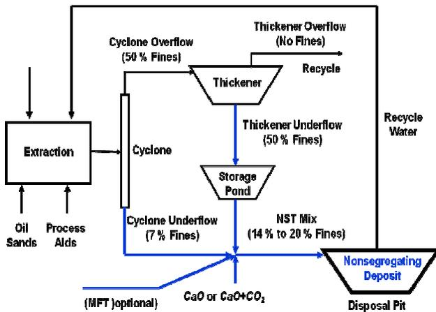
Figure 7. Production of nonsegregating tailings (NST).
