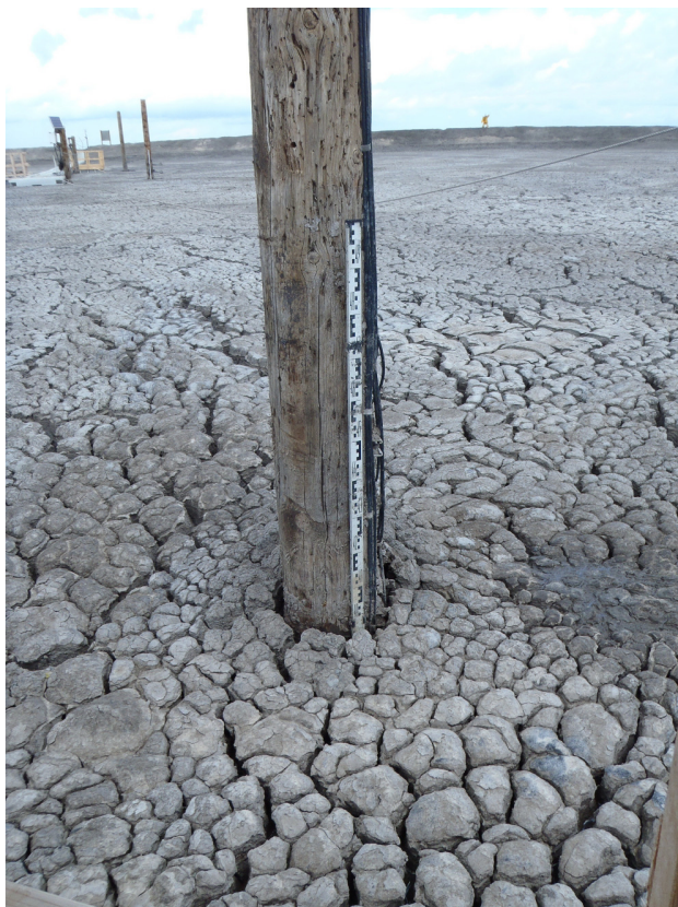
Figure 12. View of MFT surface around instrumented pole PP-3, July 6, 2010 (ten months after pit filling).
