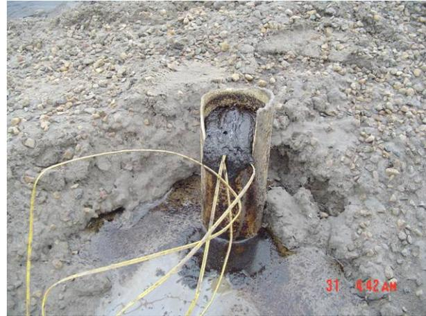
Figure 4: Bitumen flowing from PVC after blast
