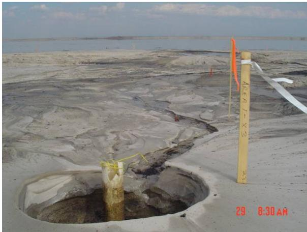
Figure 3: Erosion around PVC after blast
