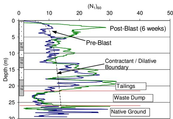
Figure 13: Area 1 (single pass) Pre- and Post-EC CPT
