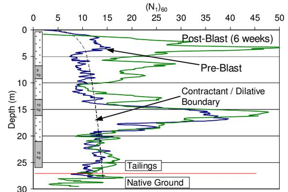
Figure 14: Area 2 (double pass) Pre- and Post-EC CPT
