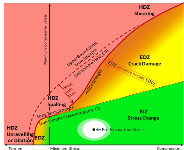
Figure 10: Damage zones mapped to the conceptual model of Diederichs (2007).
