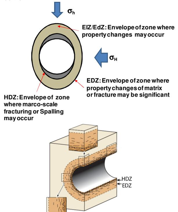
Figure 1: Illustration of the excavation damage zones for massive ground around a circular excavation. (bottom after ANDRA 2005).
