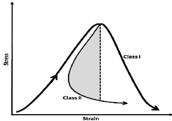
Figure 8: Stress-strain diagram showing class I and class II type post-peak behaviour for laboratory experiments as identified by Wawerik (1968) (modified from Fairhurst and Hudson, 1999).
