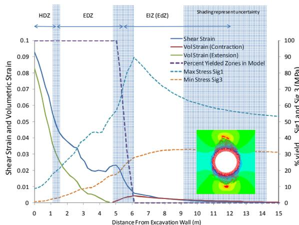
Figure 7: Example of model output using arbitrary loading and material parameters. Various indicators for EDZ and HDZ using a strain weakening model with a
