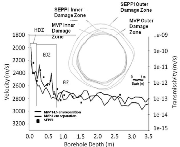
Figure 2: Changes in the velocity (MVP lines) and transmissivity (SEPPI points) with distance from the excavation face. The HDZ, EDZ, and EIZ are delineated at major changes in the slope of the graph (modified from Martino & Chandler 2004).
