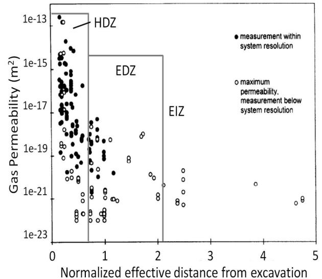
Figure 4: Gas permeabilities, measured at various locations at the WIPP project, normalized to excavation radius dimensions and EDZ dimensions indicated (modified from Stormont 1997).
