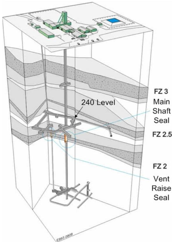
Figure 1. Layout of the URL and location of shaft seals
