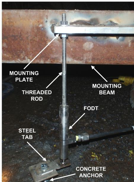
Figure 9. FODT installation detail
