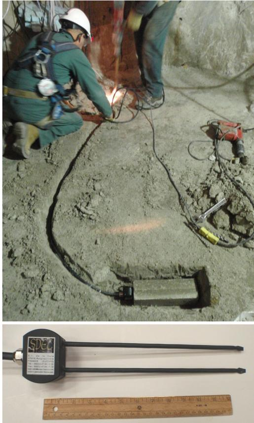
Figure 5. Installing a TDR probe in a pre-compacted bentonite-sand brick (top), TDR probe (bottom)
