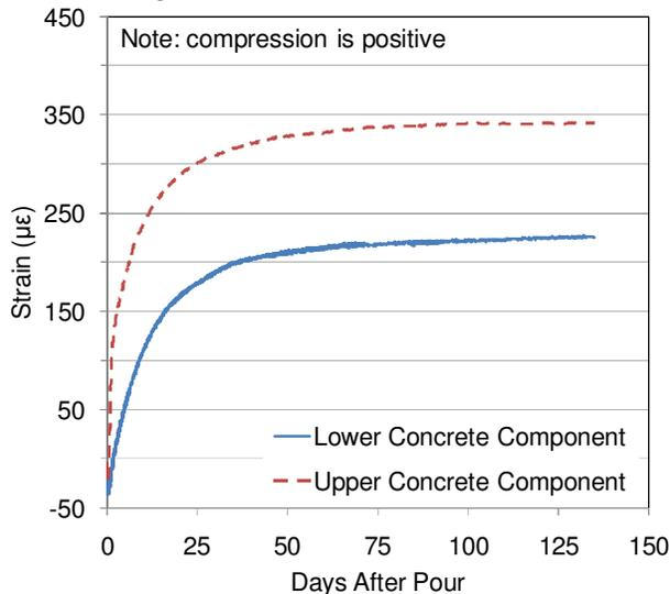
Figure 11. Average strain of the concrete components
