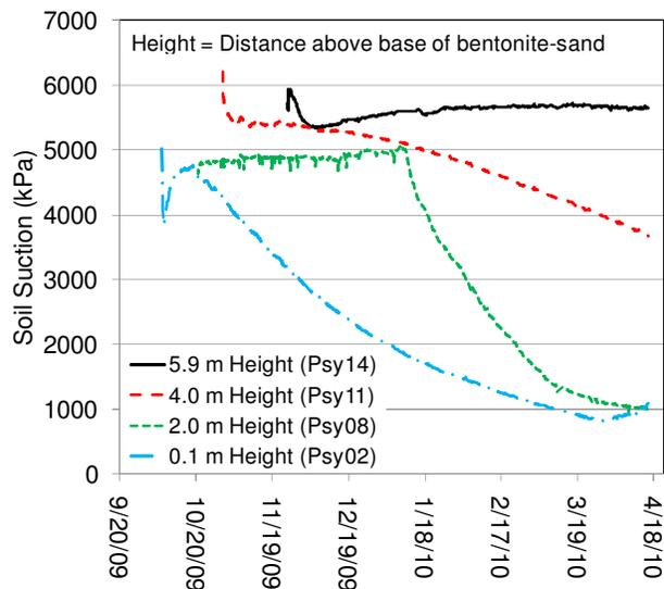
Figure 14. Soil suction in the bentonite-sand component
