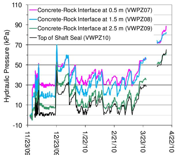
Figure 13. Hydraulic pressures at the upper concrete-rock interface and above the upper concrete component
