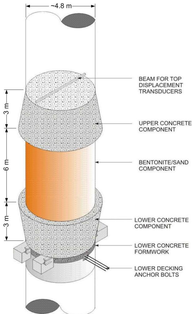
Figure 2. Schematic of the main shaft seal
