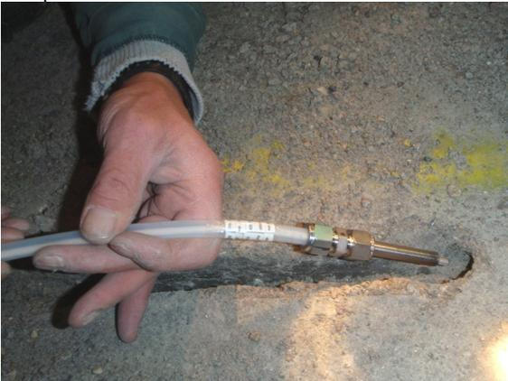
Figure 4. Installing a psychrometer in the bentonite-sand
