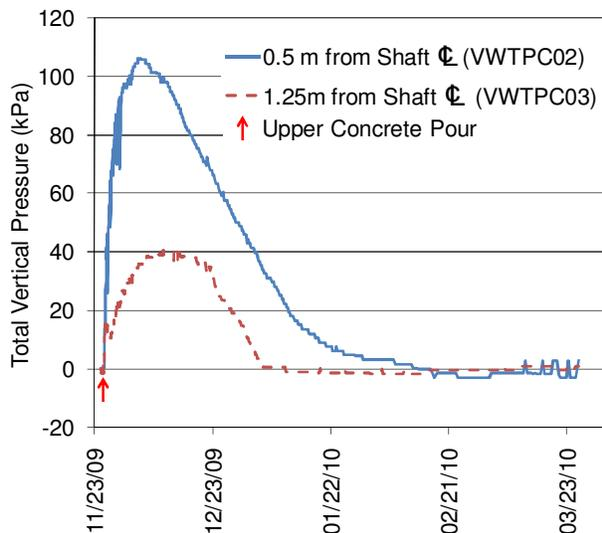
Figure 12. Total vertical pressure at the upper concrete-clay interface following the upper concrete pour
