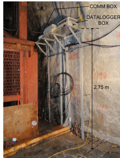
Figure 10. Sacrificial datalogger located on the 240 Level
