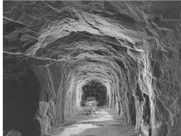
Figure 2. Raw point cloud data collected in unlined rock tunnel, 8 m diameter (Oslo, Norway).
