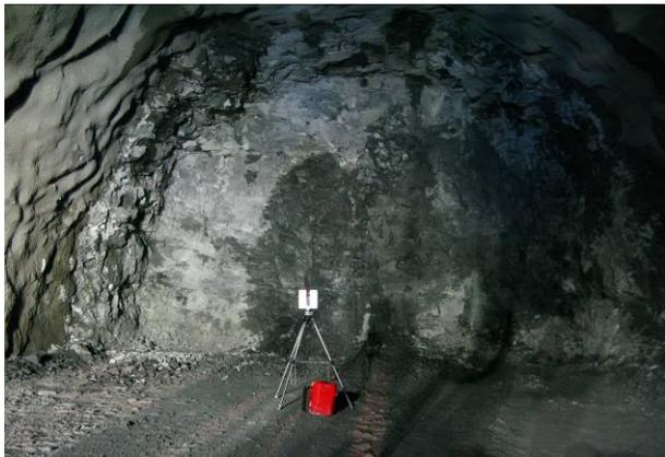
Figure 1. LiDAR data collection with tripod setup in active 10 m diameter drill and blast railway tunnel.
