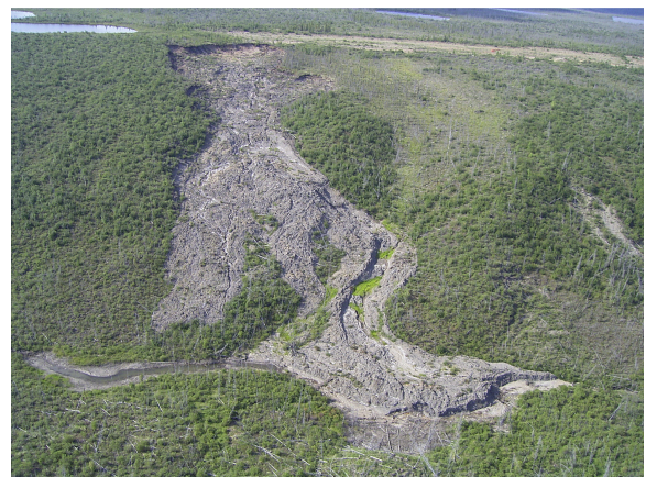
Figure 5. Retrogressive thaw flows are retrogressive, complex, slow, moist, earth slide-wet earth flows in the Working Classification (GSC-ESS Photo No. 2007-51).
