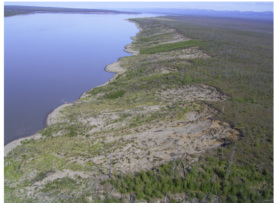
Figure 4. Example of unfrozen ground-related landslides in permafrost areas. These active layer detachments along the Mackenzie River (Northwest Territories) began in 1995 as a result of permafrost degradation due to forest fires over previous years. (GSC-ESS Photo No. 2007-41).
