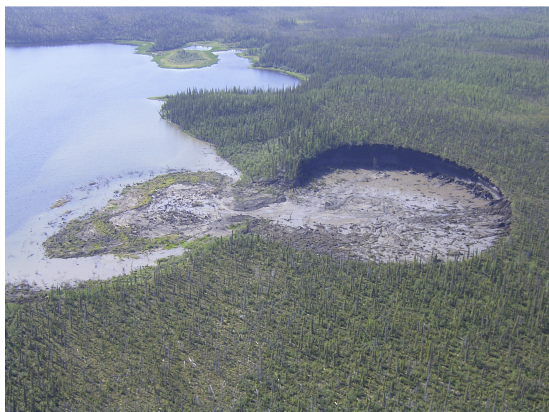
Figure 6. A bimodal flow or retrogressive thaw flow is a retrogressive, complex, slow-moderate, earth slide-very wet, earth flow in the Working Classification (GSC-ESS No. Photo 2007-59).
