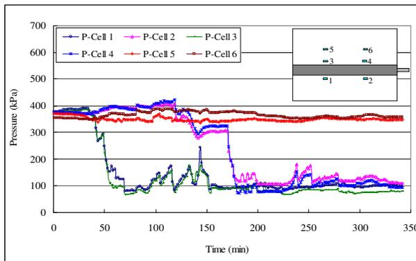
Figure 2. Relationships between earth pressures and time during drilling under overburden pressure of 350 kPa
