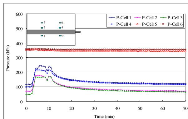
Figure 3. Relationships between earth pressures and time during pressure grouting for the tests under GP=350 kPa and OP=250 kPa.
