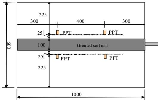
Figure 4. Locations of four pore water pressure transducers (PPT) in the soil (top view, unit: mm).
