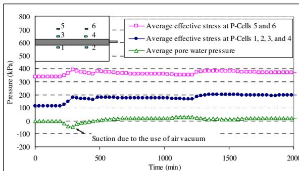
Figure 5. Variations of effective vertical stress and pore water pressure with time during the soil saturation for the test under OP = 350 kPa and GP = 250 kPa.
