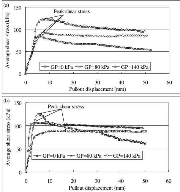
Figure 9. Development of field average shear stress of soil nails with pullout displacement when soil depth is (a) 2 m and (b) 6 m.
