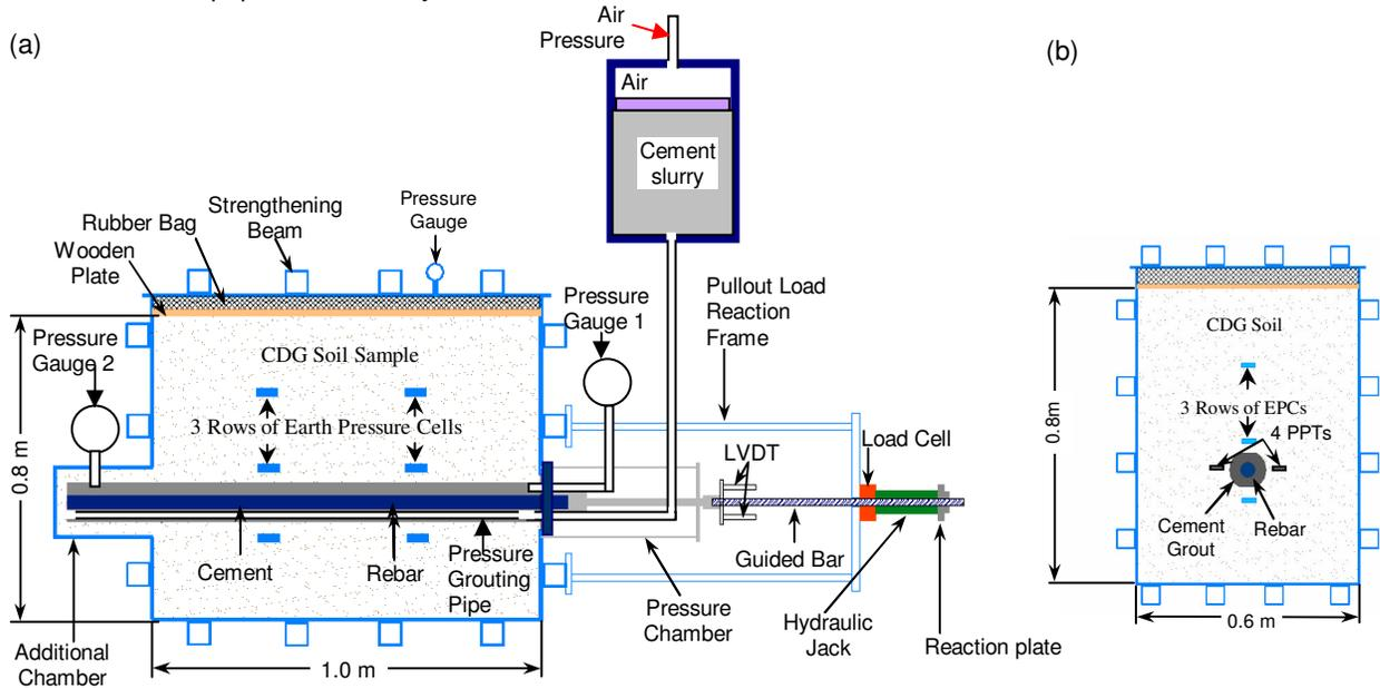
Figure 1. Set-up of the soil nail laboratory pullout test with full instrumentation and grouting and saturation devices (a) longitudinal section along soil nail, and (b) cross-section of the soil nail.
