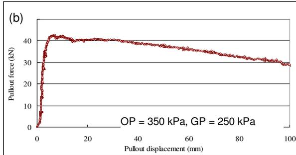
Figure 6 Monitored data during the pullout testing under OP = 350 kPa and GP = 250 kPa (a) strains at four locations in the soil nail vs. time, and (b) pullout force vs. pullout displacement
