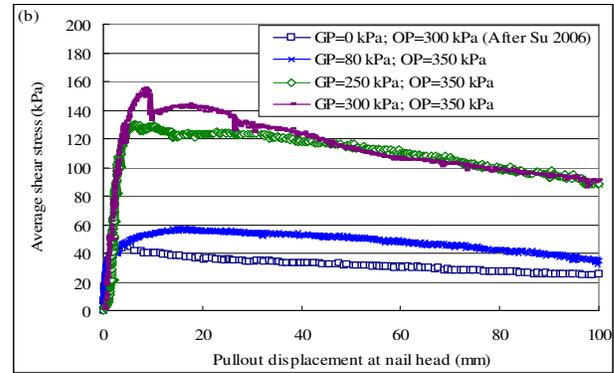
Figure 7. Variations of average interface shear stress with pullout nail head displacement under different grouting pressures (GP) and the same overburden pressure (OP): (a) GP = 130 kPa and 250 kPa, with the same OP=240 kPa (plus GP=0 kPa and OP=200 kPa from Su 2006) and (b) GP = 80 kPa, 250 kPa, and 300 kPa, with the same OP=350 kPa (plus GP=0 and OP=300 kPa from Su 2006)
