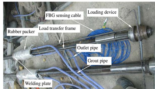
Figure 8. Full instrumentations of nail bars with fiber Bragg grating (FBG) sensors and packers before installation in drill holes.
