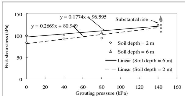
Figure 10. Peak shear stress of soil nails at different soil depths
