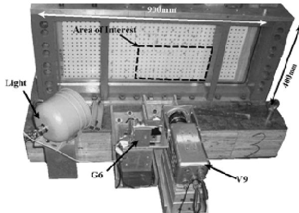
Figure 4. Location of the high-speed camera (Phantom V9) and the high-resolution still camera (Canon G6) with respect to the transparent side wall of the centrifuge test chamber. The black dots visible through the transparent window are a pre-test calibration of camera distortion through the 76 mm thick Perspex window.
