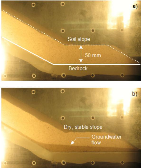
Figure 6. Photographs of toe of medium sand slope a) prior to, and b) after groundwater flow being initiated.
