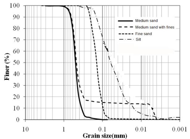
Figure 5. Grain size distribution curves for all four slope materials
