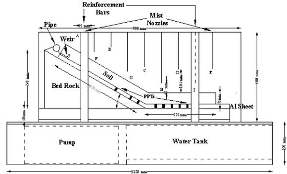
Figure 2. Test geometry
