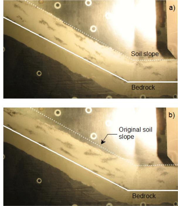
Figure 7. Photographs of toe of fine sand slope a) prior to, and b) after landsliding.
