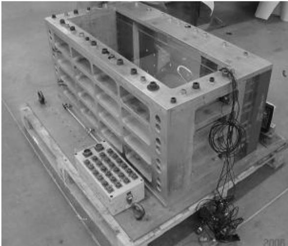
Figure 1. Plane strain testing box
