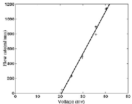
Figure 3. Calibration of flow pump at 30g
