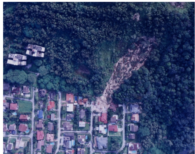
Figure 6. Debris flow from top and hit damage the bungalow
