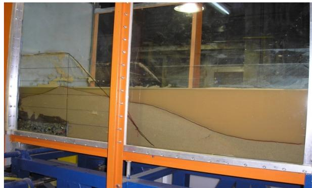
Figure 9. Final slope at the end of Test No. 2
