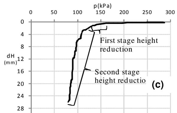
Figure 2. Behavior of Firoozkooh No. 151 sand in CDS loading (modified after Azizi and Imam 2008)
