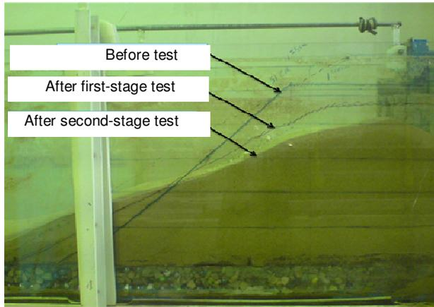
Figure 7 Locations of the slopes before the test and at the end of the first and second stages of Test No. 1
