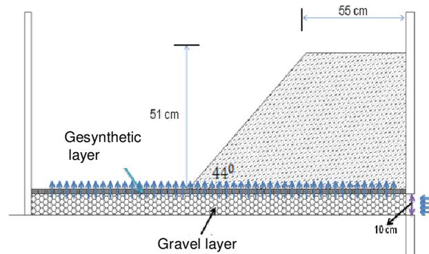
Figure 6. Geometry and slope for Test No. 1
