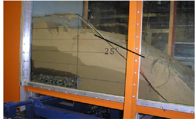
Figure 8. Slope after first collapse in Test No. 2
