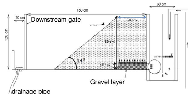
Figure 3. Schematic figure of the tank in one of the tests
