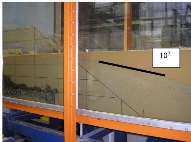
Figure 12. Final condition of the slope in Test No. 3. Outline of the slope initial condition is also shown.
