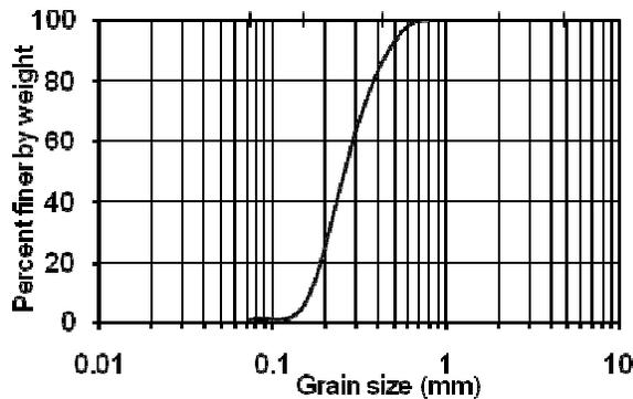
Figure 1 – Grain size distribution of Firoozkooh No. 151 sand
