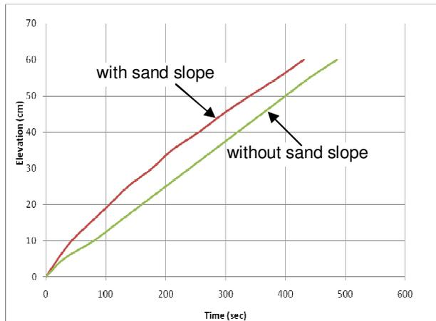
Figure 5. Changes in the water level elevation with time in the tank with and without the sand slope
