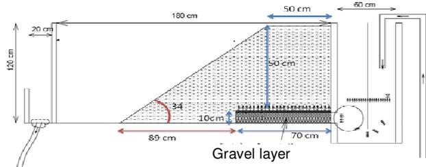
Figure 10. Geometry and slope for Test No. 3
