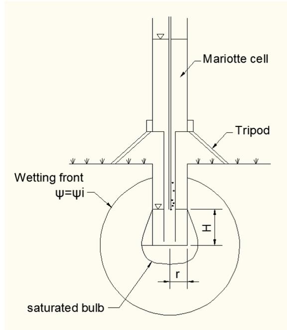
Figure 1 : Schematics of the Guelph permeameter and water occurrences in the infiltration zone
