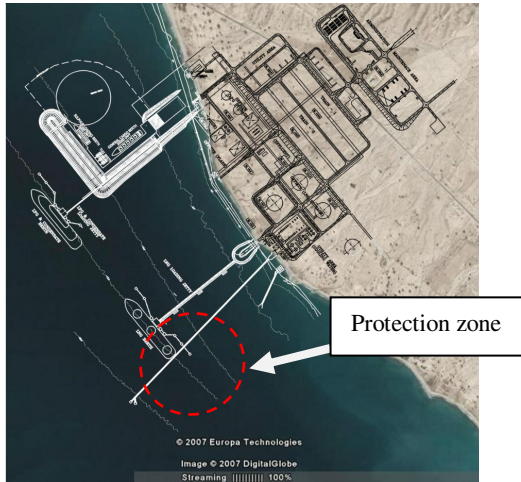
Figure 2. General layout of the LNG port
