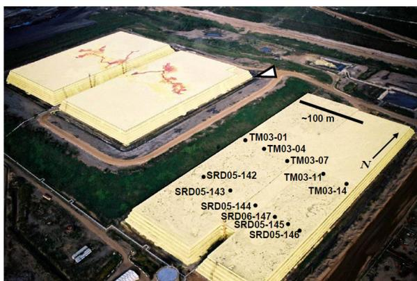
Figure 1. Aerial photo of Phase 1 (lower right) and 2 (upper left, under construction)  $S^0$  blocks at Syncrude Canada Ltd. oil sands mine in 2003. Black dots on the Phase 1 block represent locations of vertically-nested gas sampling ports (SRD series) and thermistors (TM series). The white triangle at the north-east corner of the Phase 2 block represents the location of the weir and drainage sampling location. The dark texturing on the surface of the Phase 1 block is wind-blown sediment.
