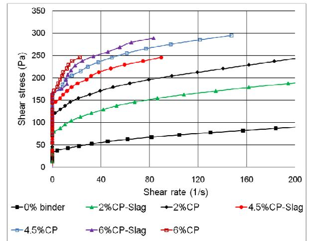
Figure 9: Flow curves for TT and CPB samples at 2 hours curing time for different contents of binder types CP and CP-Slag.
