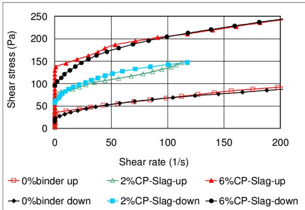
Figure 5: Up and down flow curves of CPB with 2 wt% and 6 wt% of GU-Slag binder type using a linear plotting scale at 0 h curing time.
