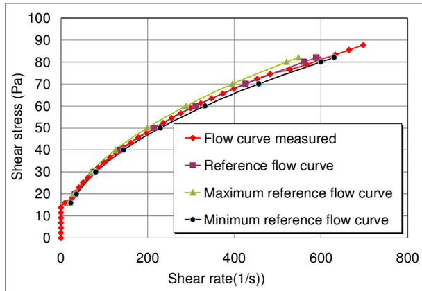
Figure 3. Reference and measured flow curves of certified non-Newtonian fluid NNTF1
