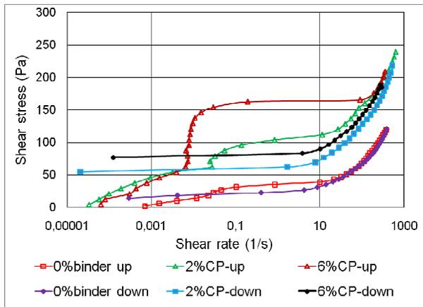
Figure 6: Up and down flow curves of CPB with 2 wt% and 6 wt% of CP binder type using a semi-logarithmic scale at 0 h curing time.
