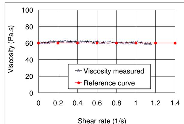
Figure 2. Viscosity curves of certified Newtonian fluid RT 60000 fluid
