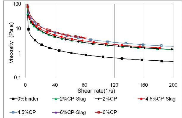
Figure 13. Viscosity curves for CPB at 4 hours curing time for different contents of binder types CP and CP-Slag.
