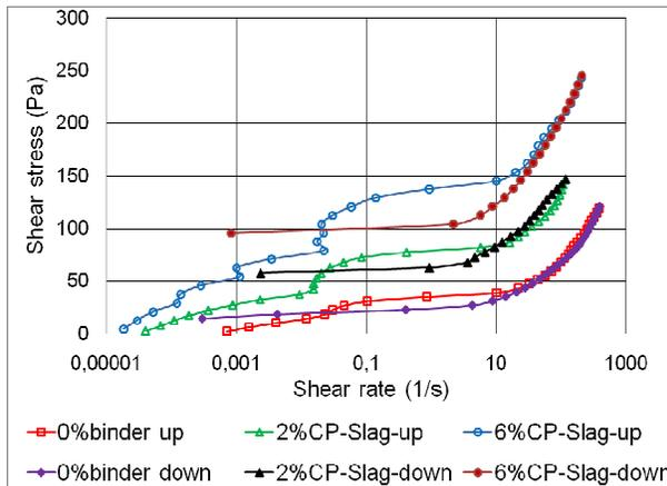
Figure 7: Up and down flow curves of CPB with 2 wt% and 6 wt% CP-Slag binder type on semi-logarithmic scale at 0 curing time.
