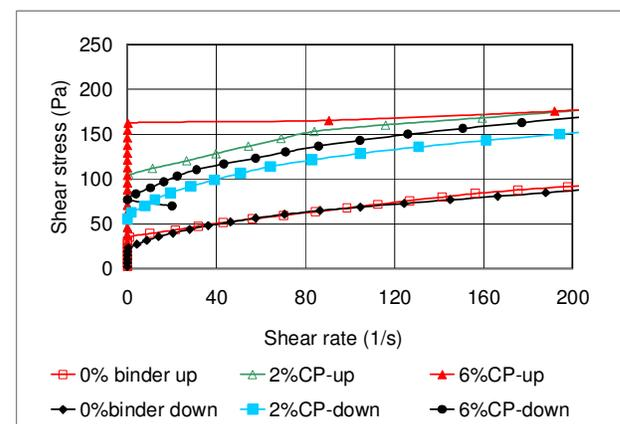
Figure 4. Up and down flow curves for CPB samples with 2 wt% and 6 wt% of CP binder type using a linear scale at 0 h curing time.
