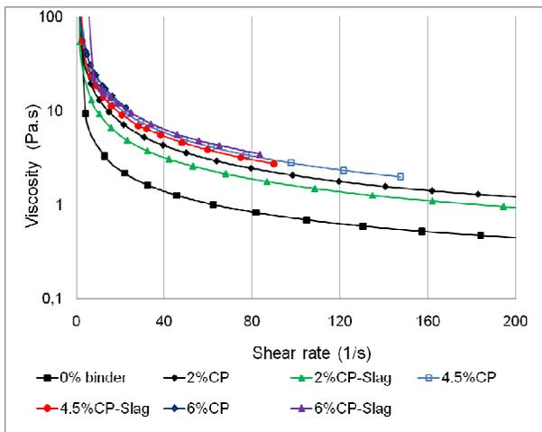
Figure 12. Viscosity curves for TT and CPB samples at 2 hours curing time for different contents of binder types CP and CP-Slag.
