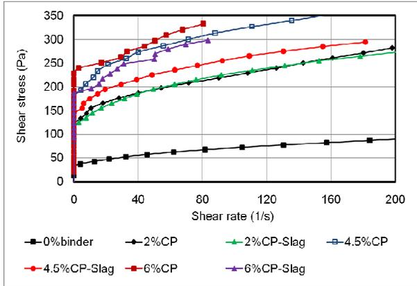
Figure 10. Flow curves for CPB samples at 4 hours curing time for different contents of binder types CP and CP-Slag.
