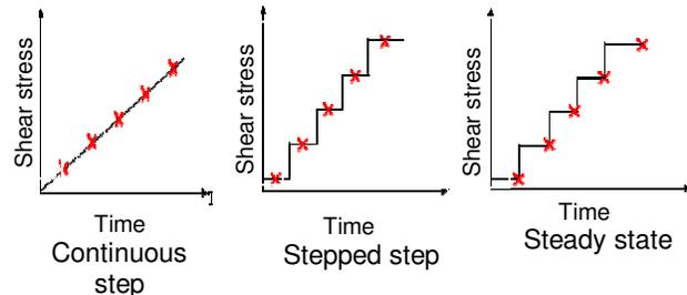
Figure 1. Shearing procedures using the AR 2000 torsional rheometer (crosses indicate rheological parameter sample points).
