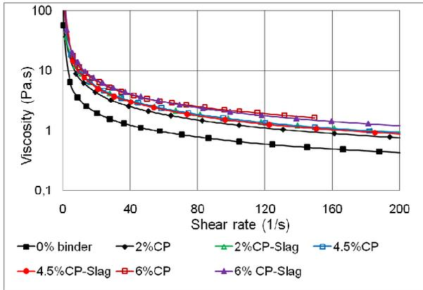
Figure 11. Viscosity curves for TT and CPB samples at 0 hour curing time for different contents of binder types CP and CP-Slag.
