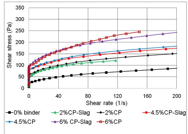
Figure 8: Flow curves for TT and CPB samples at 0 hour curing time for different contents of binder types CP and CP-Slag.
