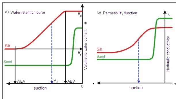
Figure 1 : Schematic view of typical water retention curves and permeability functions for a sand and a silt (adapted from Aubertin et al., 1995)
