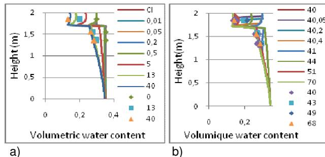
a) Figure 8 : Experimental results (dots) and numerical simulations (lines) for the first (a) and second cycles (b) of drainage; the results are presented in terms of volumetric water content ( $\theta$ ) at different times (in days).
