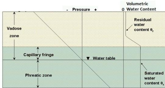
Figure 3 : Schematic view of the volumetric water content and pore water pressure equilibrium distribution above the water table in homogeneous tailings (adapted from MEND, 1996)
