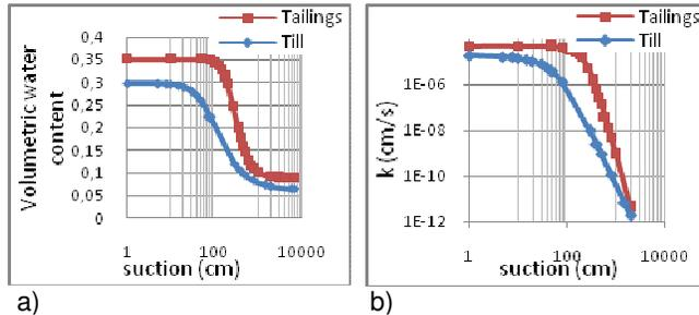
a) Figure 7 : Water retention curves (a) and  $k_r$  functions (b) of the tailings and till; these adjusted functions are used for the basic numerical model calculations.
