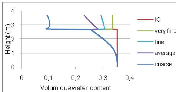
Figure 12 : Volumetric water content profiles for the four types of cover material (shown after 56 days of drainage)
