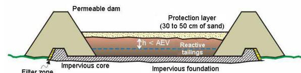
Figure 2 : Conceptual model of the elevated water table technique implemented with a monolayer cover placed over reactive tailings (adapted from Aubertin et al., 1999).
