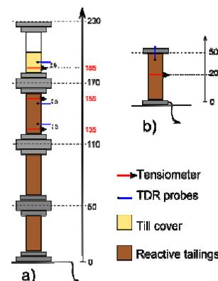
Figure 4 : Representation of the instrumented large (a) and small (b) columns.
