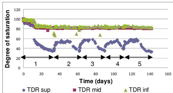
Figure 5 : Degree of saturation values in the large column SG1 for the first five drainage cycles
