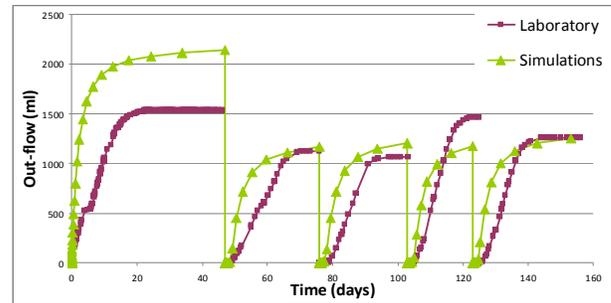
Figure 9 : Evolution of the cumulated outflow at the base of column SG1 measured in the laboratory (red) and obtained from the simulations (green).
