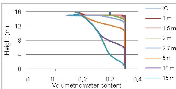
Figure 13 : Volumetric water content profiles for the seven values imposed for the water table depth (shown after 56 days of drainage)
