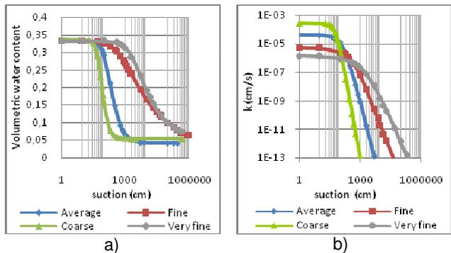
Figure 11 : WRCs (a) and the  $k_u$  functions (b) for the cover materials introduced in the simulations with SEEP/W
