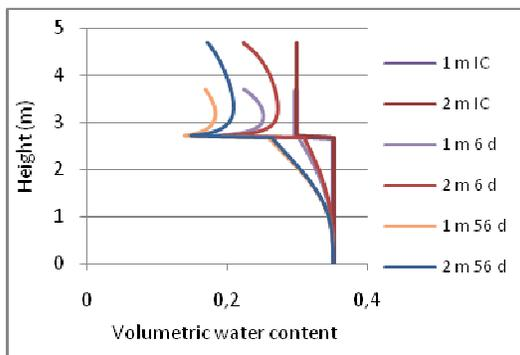
Figure 10 : Volumetric water content profiles for the two cover thicknesses at different times (in days)
