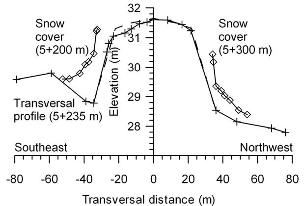
Figure 8. Elevation of the embankment surface on July 2004 and snow surface on April 2005 on the Southeast and Northwest shoulders and toes of the airfield embankment at Tasiujaq Airport, Northern Quebec, Canada. The dash line is the transversal profile as built (MTQ 1990). Note the vertical exaggeration 1:40.
