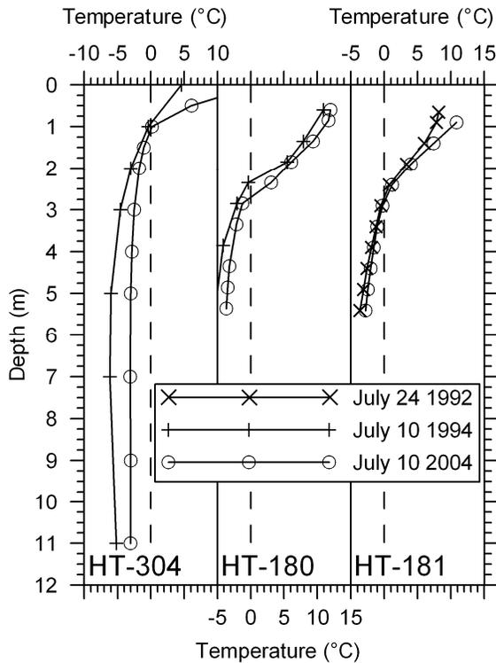
Figure 6. Temperature profiles in the field (HT-304) and in the airfield embankment and subgrade (HT-180 and HT-181) at Tasiujaq Airport, Northern Quebec, Canada. See Figure 3 for the location of thermistor cables HT-304, HT-180 and HT-181.
