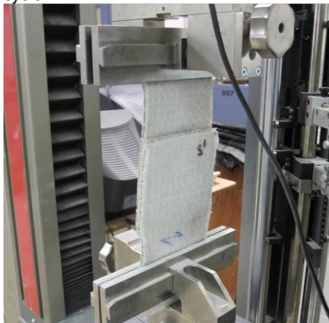
Figure 5. Photograph of GCL overlap sample in prior to the start of a test.
