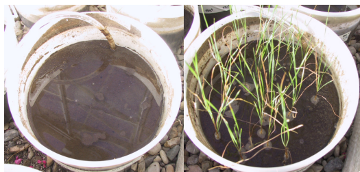
Figure 4 Free water in unplanted sample and plant channels in planted samples
