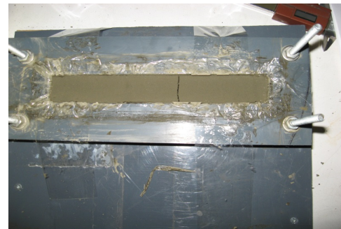
Figure 10. Crack on the tailings specimen during the restrained desiccation test on the Bulyanhulu tailings.
