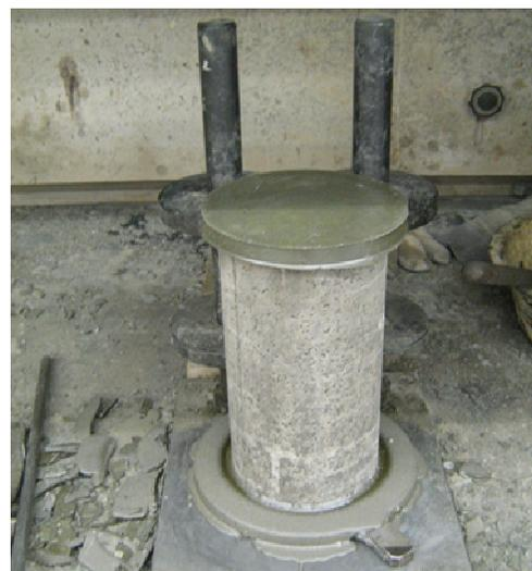
Figure 5. Photo showing the capping process prior to UCS testing
