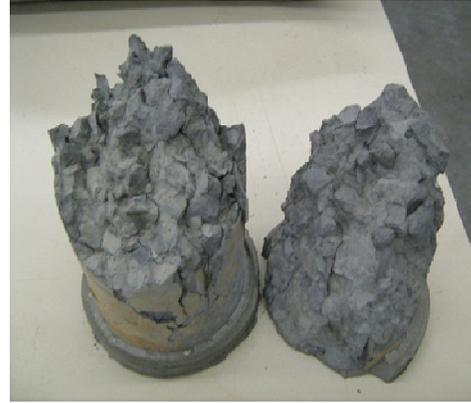
Figure 7. Photos showing the breaking pattern of a composite concrete specimen after 14 days of curing
