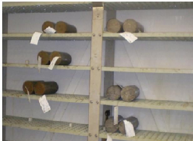
Figure 3. Specimens curing in the humidity chamber
