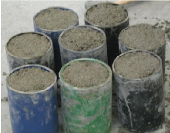
Figure 2. Photos showing cast plastic moulds
