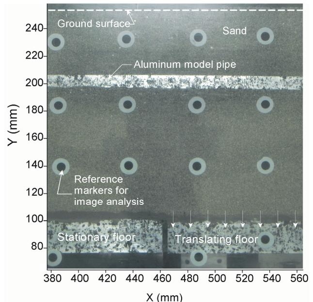
Figure 5. Digital photograph from central view of the test model before starting the test
