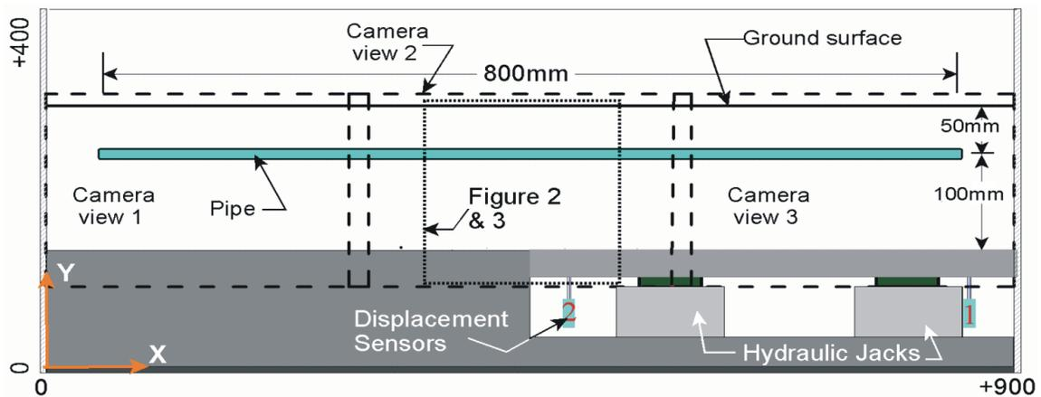
Figure 1. Test geometry (vertical section through the front face of the test box, parallel to the axis of the half-pipe).
