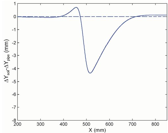
Figure 8. Distribution along the pipe of vertical pipe displacement relative to the soil
