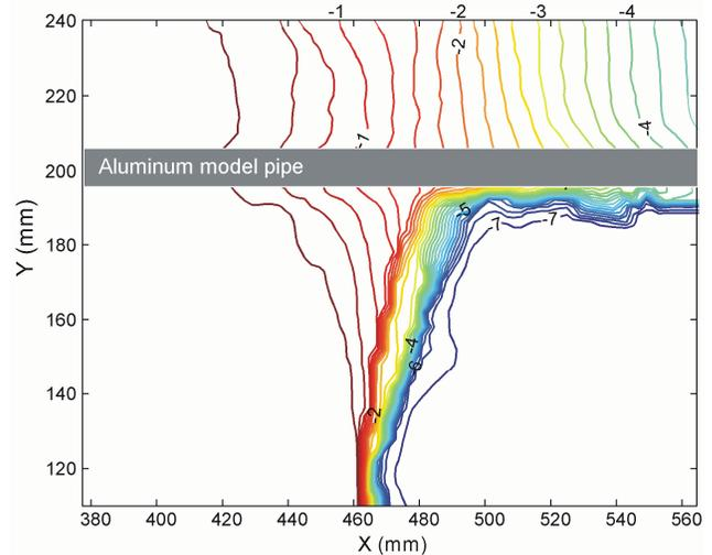
Figure 4. Soil displacement contours for the test with half-pipe
