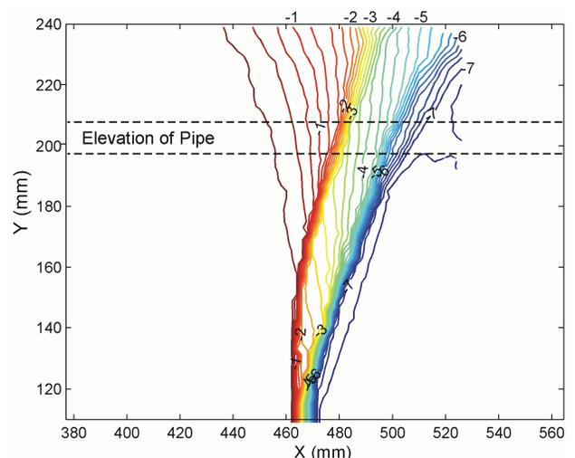
Figure 2. Soil displacement contours for the test without the half-pipe
