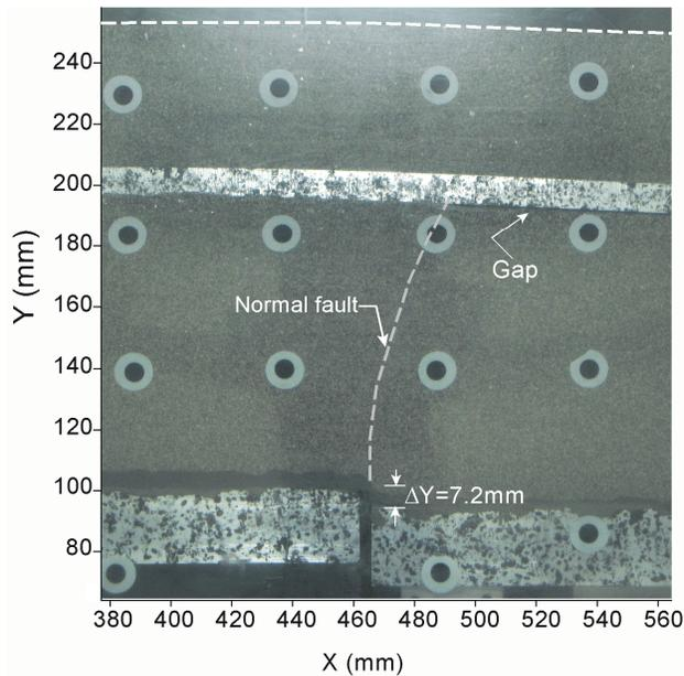
Figure 6. Digital photograph from central view of the test model after the test
