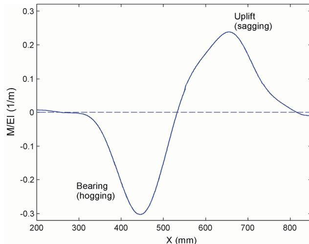
Figure 9. Bending moment distribution along the pipe (model scale)
