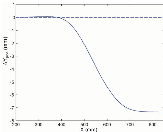
Figure 7. Distribution of vertical pipe deflections along the pipe
