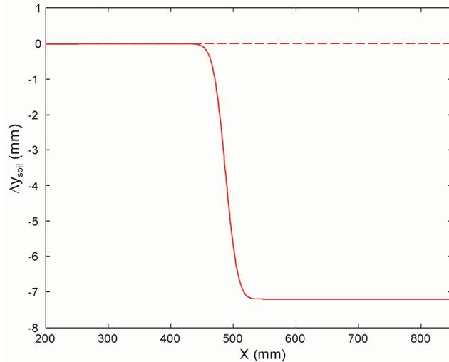
Figure 3. Soil displacements at pipe elevation in free field test
