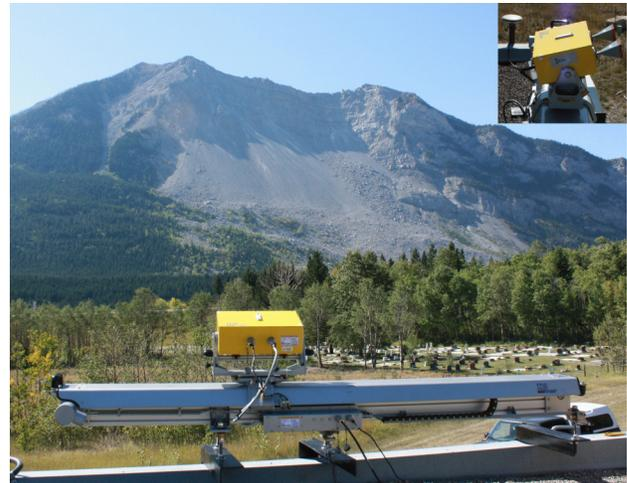
Figure 2. The IBIS-L GB-InSAR system is installed on a rooftop, facing unstable slopes on Turtle Mountain. The farthest point on the mountain crest is approximately 3200 metres away.
