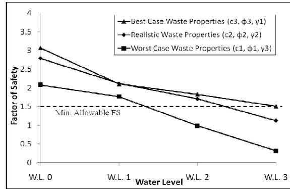
Figure 5. Safety factor for four water level scenarios
