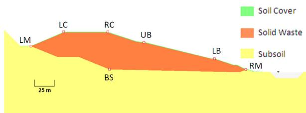
Figure 1. Cross-section of the Advance Phase of Bukit Tagar Landfill
