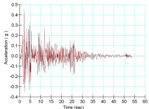
Figure 4. Modified time-history of El Centro earthquake used for seismic analysis
