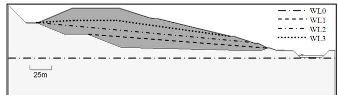
Figure 2. Water level scenarios used for simulations
