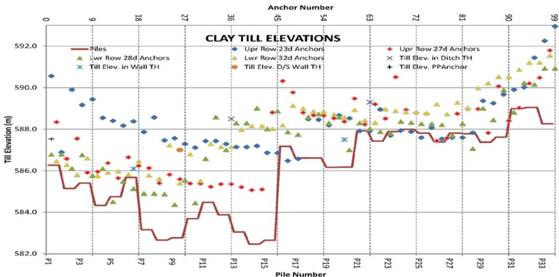
Figure 5. Clay Till and Anchor Bond Zone Elevations along Upper Wall
