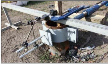
Figure 8: Lateral load setup: steel clamp/LVDT plate
