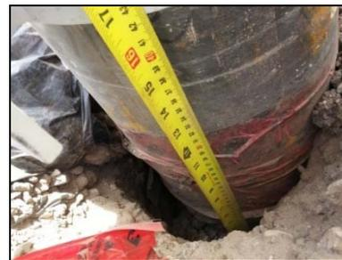
Figure 13: An image of the developed gap behind pile PC1 at the end of the cyclic lateral testing
