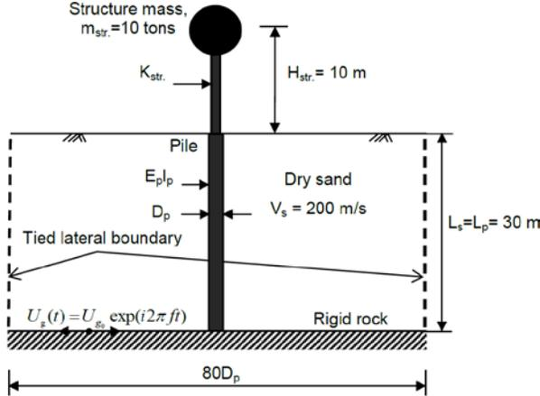
Figure 1. Basic characteristics of the SPS system under investigation and associated boundary conditions.
