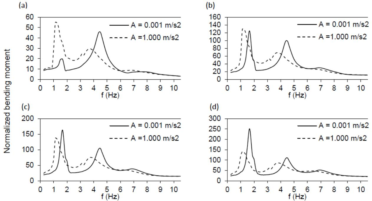
Figure 3. Effect of nonlinearity on maximum normalized seismic kinematic bending moment amplitude (at the most adverse location along the pile) for inhomogeneous soil layer and: (a)  $S_H=1.78$ , (b)  $S_H=3.56$ , (c)  $S_H=4.23$ , and (d)  $S_H=6.32$ .
