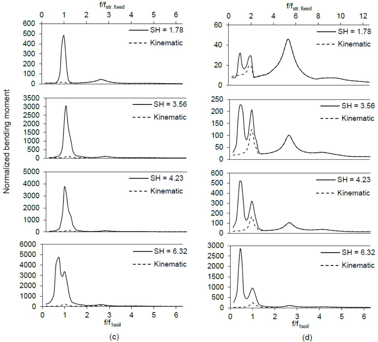
Figure 2. Maximum normalized bending moment amplitude (at the most adverse location along the pile) for homogeneous soil layer ( $A = 0.001\text{m/s}^2$ ) and: (c)  $(1/\sigma) = 0.10$  and (d)  $(1/\sigma) = 0.04$ .
