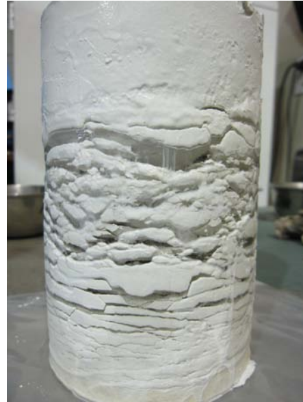
Figure 8. Close Up Photograph of Ice Lenses at End of Test
