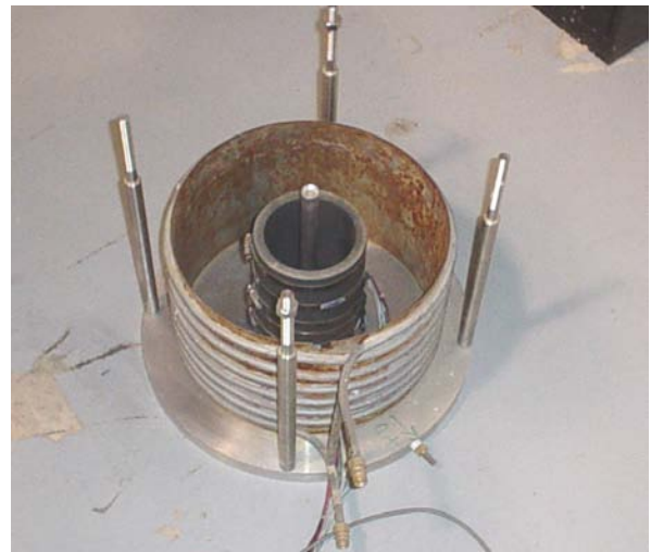
Figure 2. Cell Barrel Inside Temperature Control Jacket
