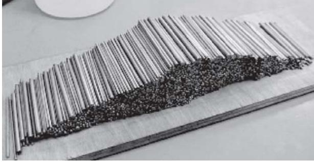
Figure 7. Material used in 2D model tests (Nakai 2013)
