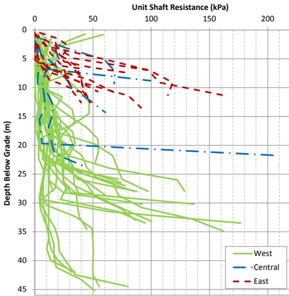
Figure 11. Unit shaft resistance (kPa) from CAPWAP.
