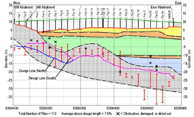
Figure 9 Variations in installed pile lengths.
