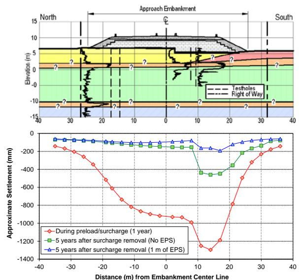
Figure 6. East approach fill with expanded polystyrene lightweight fill, soil profile and predicted settlement.
