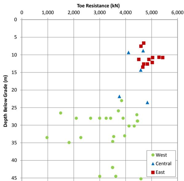
Figure 12. Unit toe resistance (kPa) from CAPWAP.
