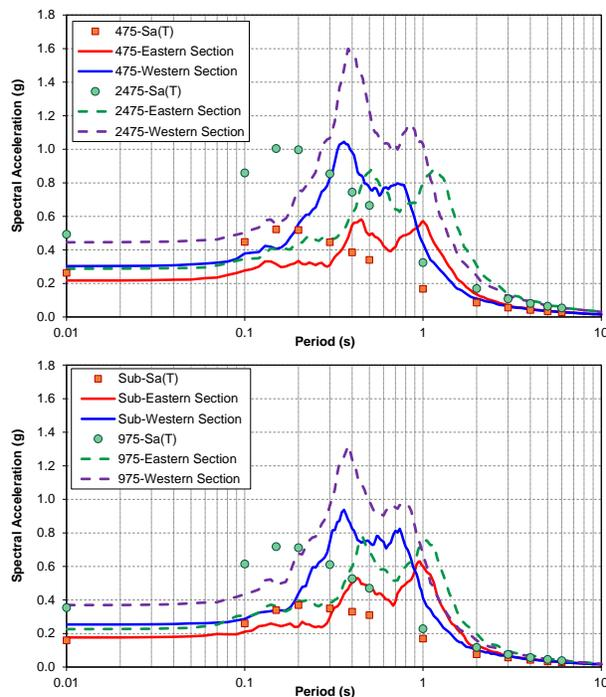
Figure 5. Structural response spectra for the eastern and western sections of the bridge structure
