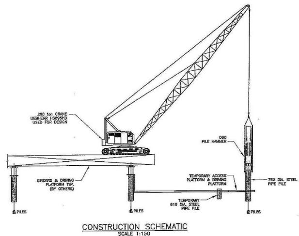
Figure 3. Top-Down construction schematic
