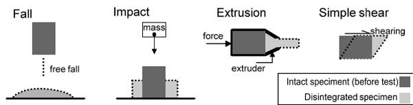
Figure 5. Schematic illustration of processes responsible for the disintegration of sensitive clays involved in a landslide as studied by Tavenas et al. (1983)
