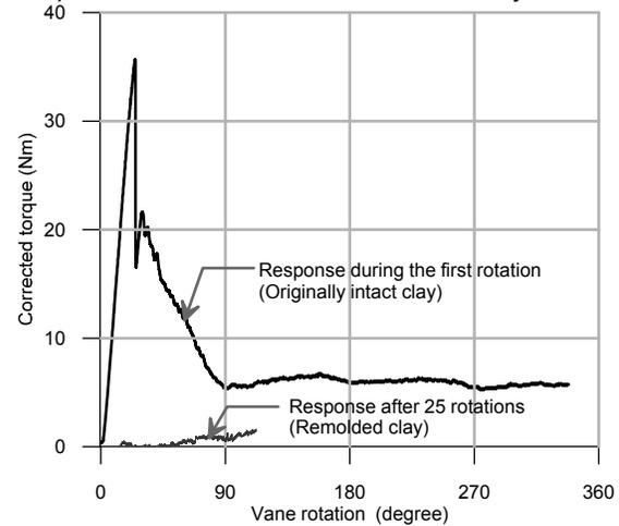
Figure 8. Typical vane shear test result
