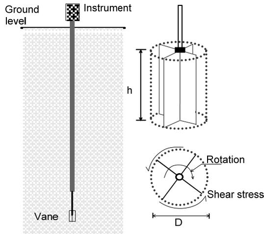
Figure 7. Vane shear apparatus
