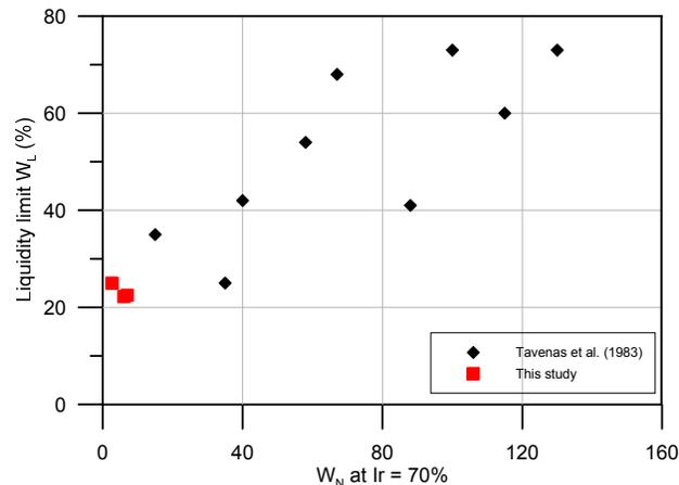
Figure 14. Disintegration energy at  $I_r = 70\%$  as a function of liquid limit
