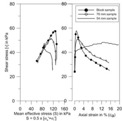
Figure 3. Effect of sample disturbance in sensitive clays taken from 10m depth. Here  $\sigma'_a$  and  $\sigma'_r$  are the effective stresses in the axial and the radial direction, respectively. The presented results are from the Kløfta road project in Norway (Source; NPRA, 2009)
