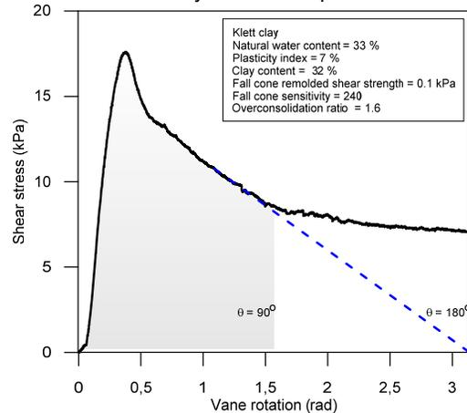
Figure 11. Shear stress-vane rotation curve for the tested Klett sensitive clay at 8.5 m depth
