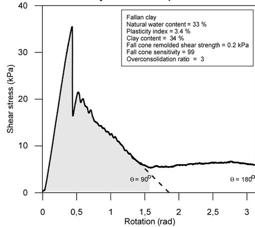
Figure 10. Shear stress-vane rotation curve for the tested Fallan sensitive clay at 8.5 m depth
