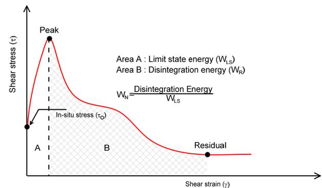
Figure 4. Illustration of disintegration energy concept
