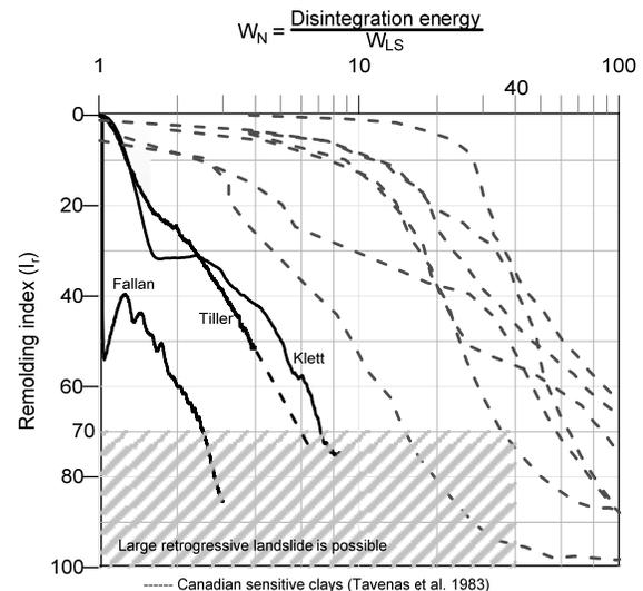
Figure 13. Remolding energy vs remolding index
