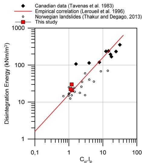
Figure 15 Disintegration energy of the Norwegian and Canadian clays
