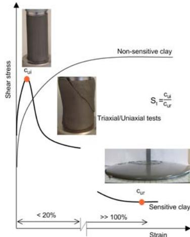
Figure 2. Schematic representations of a soft sensitive clay subjected to deformation; from the intact and the fully disintegrated (remolded) state. (Thakur and Degago, 2014)
