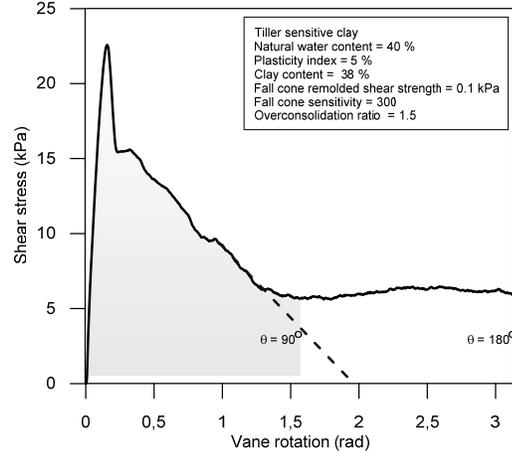
Figure 9. Shear stress-vane rotation curve for the tested Tiller sensitive clay at 8.5 m depth
