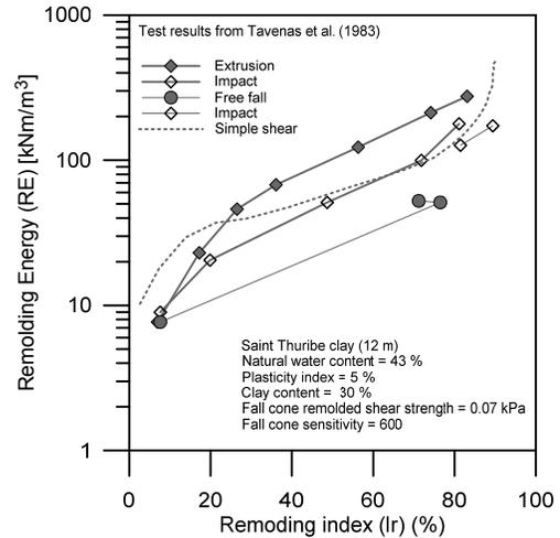
Figure 6. Disintegration energy at different level of disintegration of the Saint-Thuribe specimen tested using different techniques based on the laboratory observation by Tavenas et al. (1983)
