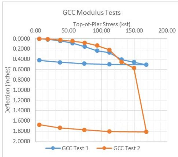
Figure 9. GeoConcrete Column Modulus Test Results
