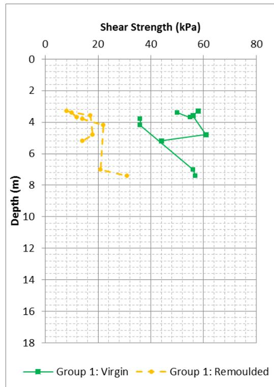
Figure 2. Pre-installation undrained shear strength vs. depth for Group 1
