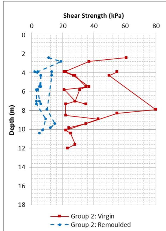
Figure 4. Pre-installation undrained shear strength vs. depth for Group 2
