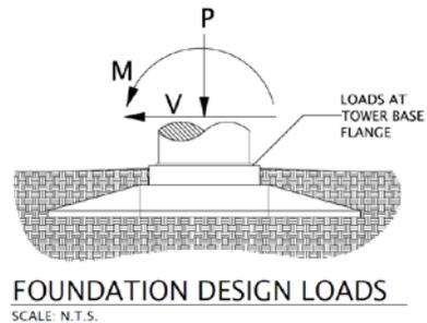
Figure 5. Typical Forces and Moments at a Wind Tower
