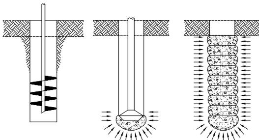
Figure 6. Installation process of the GP3® System
