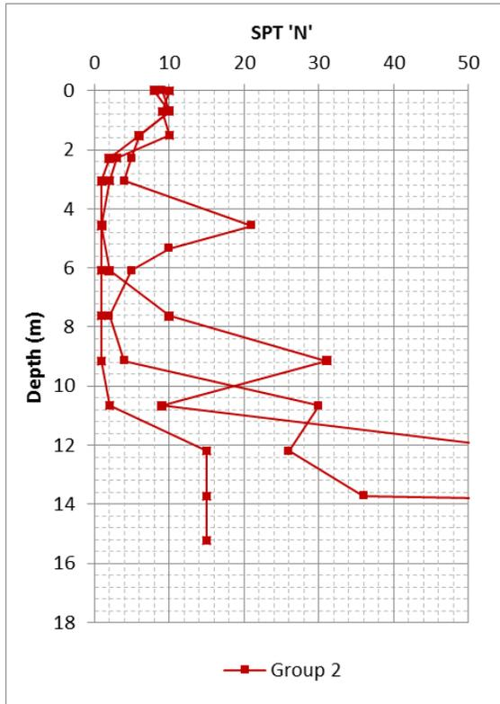
Figure 3. Pre-installation SPT 'N' values vs. depth for Group 2
