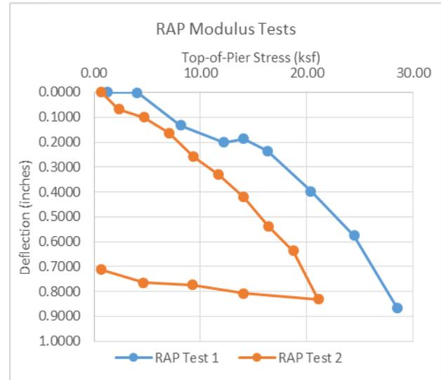
Figure 8. Rammed Aggregate Pier Modulus Test Results
