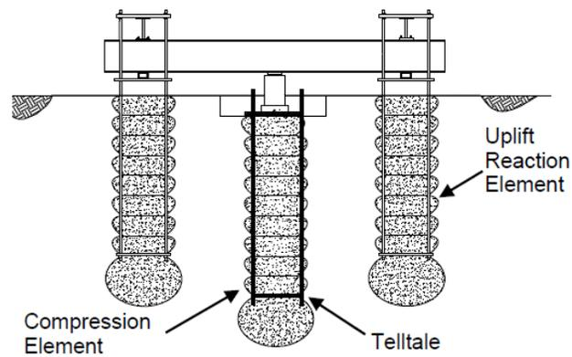
Figure 7. Full scale modulus test setup
