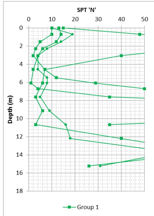
Figure 1. Pre-installation SPT 'N' values vs. depth for Group 1
