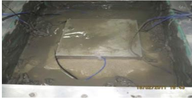
Fig. 4. Observed Uplift of structure model (Zhou et al. 2015)
