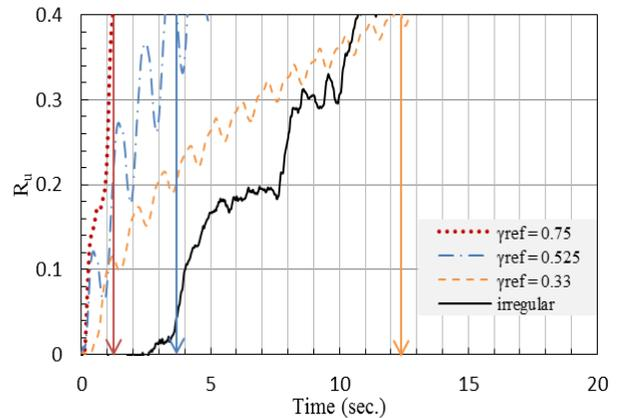
Figure 10. Pore pressure buildup and number of cycles required to cause  $R_u = 0.4$  at Freq.=1Hz.
