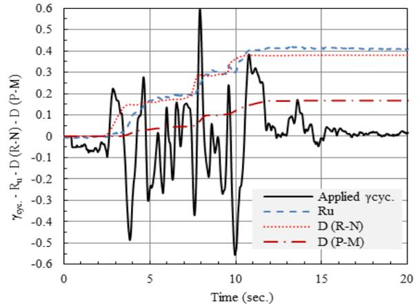
Figure 8. Relation between non-uniform shear strain  $\gamma_{cyc}$ ,  $R_u$ , cumulative damage by P-M and R-N hypotheses for Baie Saint-Paul Sand.
