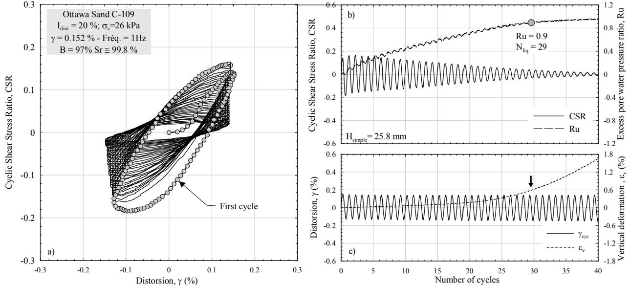
Figure 3. Typical records of  $T_{xSS}$  test on Ottawa C-109 sand
