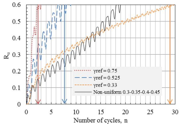
Figure 9. Pore pressure buildup and number of cycles required to cause  $R_u = 0.6$  at Freq.=1 Hz.
