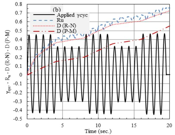
Figure 7. Relation between applied  $\gamma_{cyc}$ ,  $R_u$ , cumulative damage computed by P-M and R-N hypotheses for Baie Saint-Paul Sand.
